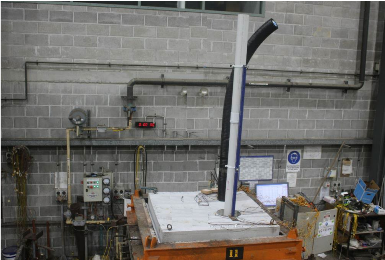
PHOTOGRAPH 3 – UNEXPOSED FACE OF SPECIMENS PRIOR TO TESTING
