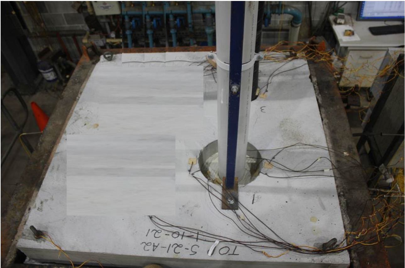
PHOTOGRAPH 4 – UNEXPOSED FACE OF SPECIMENS PRIOR TO TESTING
