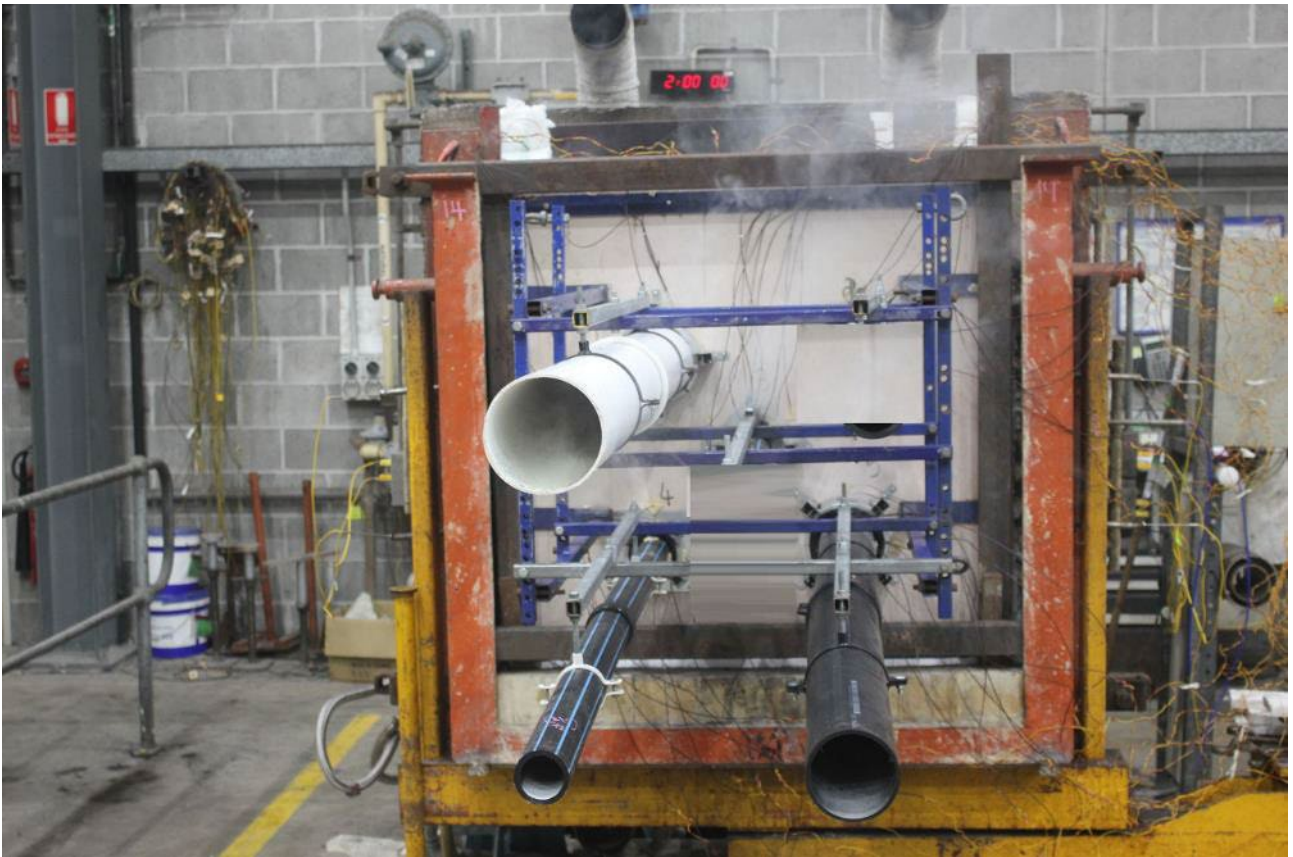
PHOTOGRAPH 9 –SPECIMENS AFTER 120 MINUTES OF TESTING
