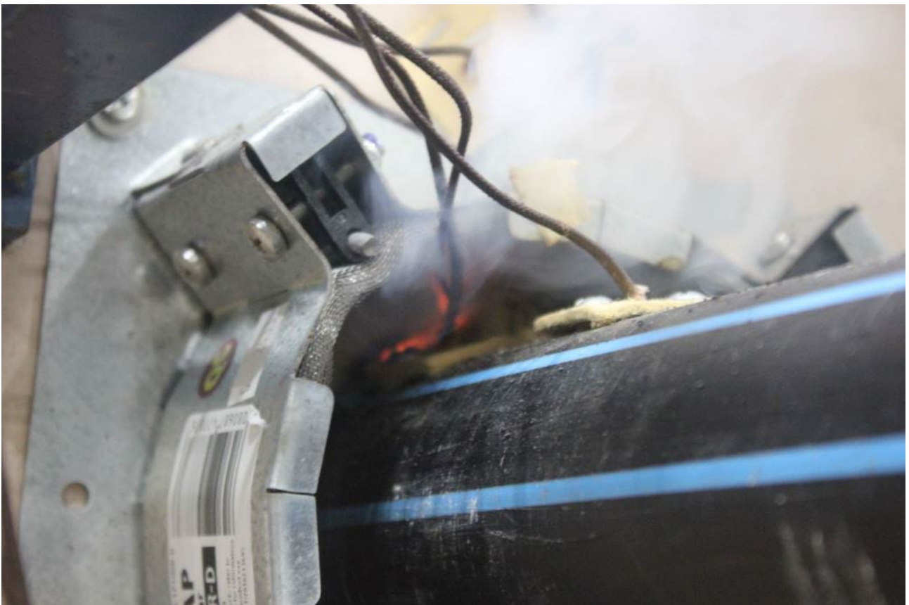
PHOTOGRAPH 10 –SPECIMEN 4 AFTER 147 MINUTES OF TESTING
