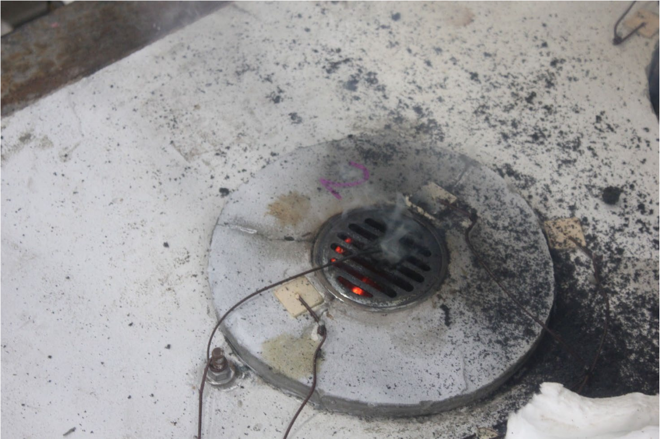
PHOTOGRAPH 15 – SPECIMEN 2 AT 185 MINUTES INTO THE TEST.
