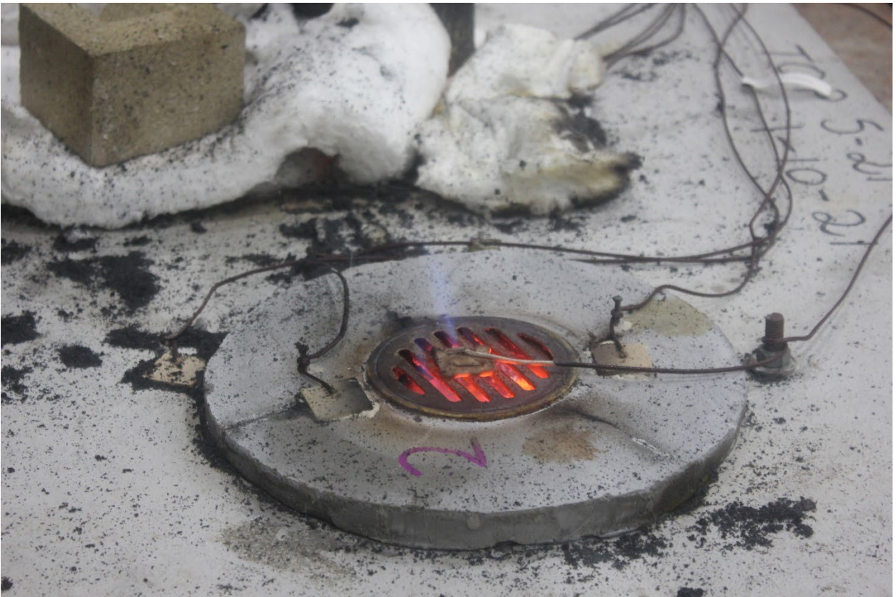
PHOTOGRAPH 17 – SPECIMEN 2 AT 211 MINUTES INTO THE TEST
