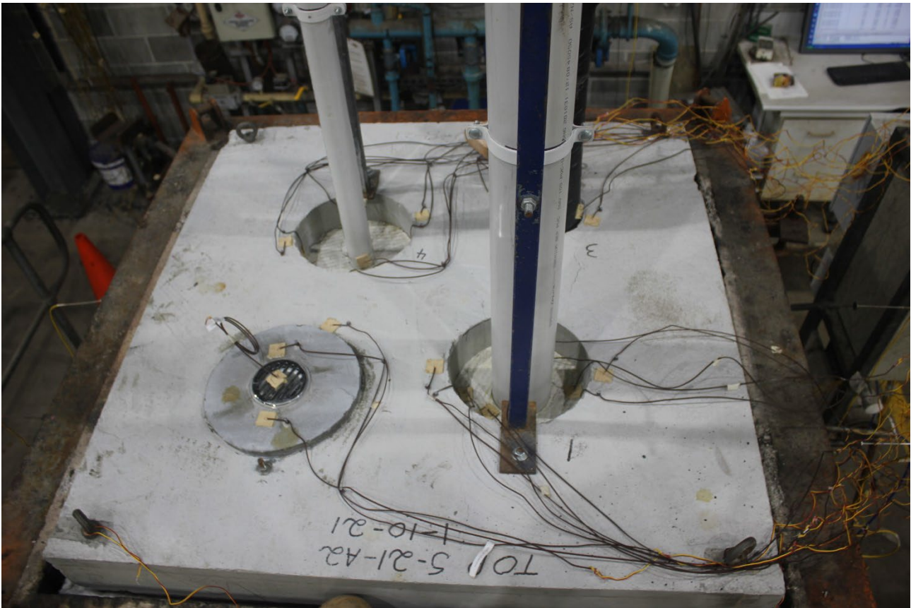
PHOTOGRAPH 3 – UNEXPOSED FACE OF SPECIMENS PRIOR TO TESTING
