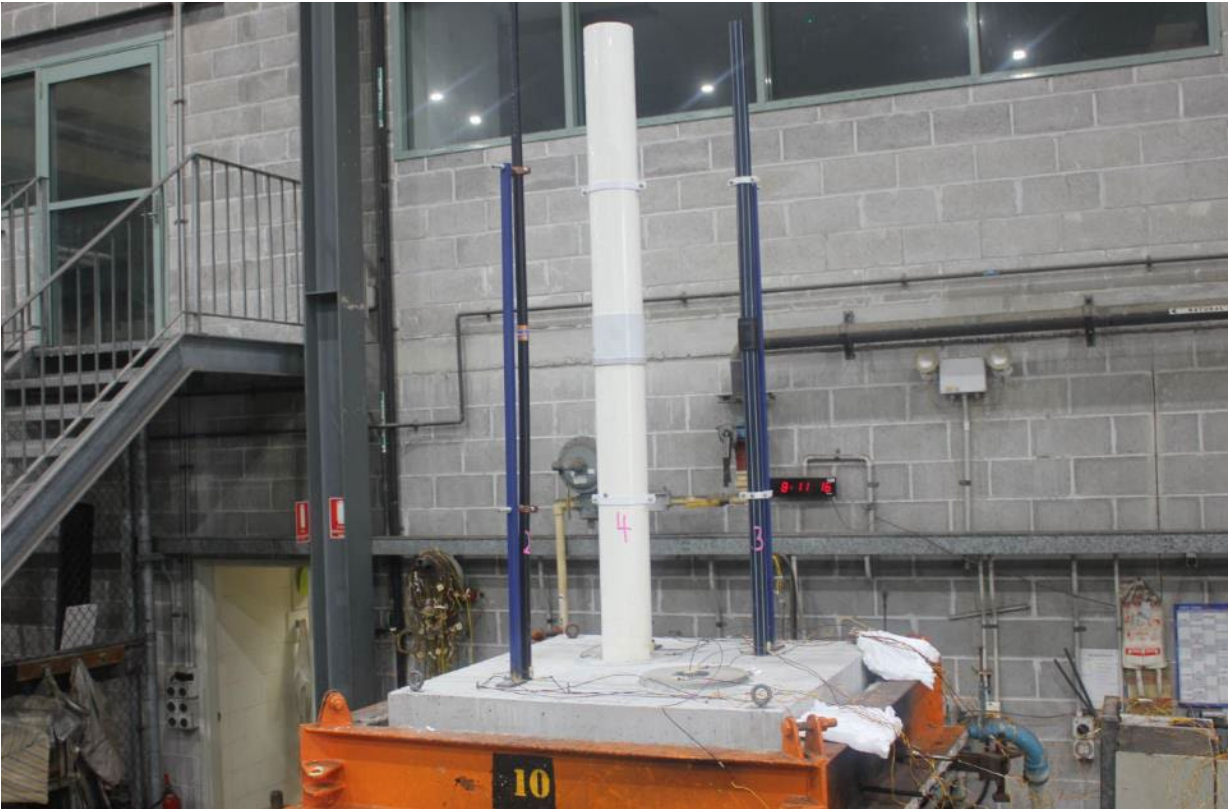
PHOTOGRAPH 2 – UNEXPOSED FACE OF SPECIMENS PRIOR TO TESTING
