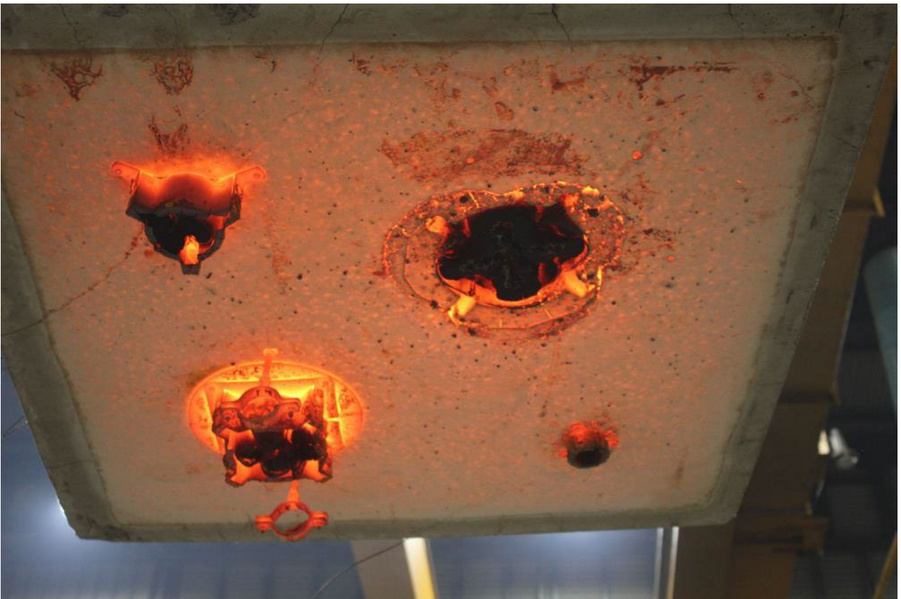
PHOTOGRAPH 14 – EXPOSED FACE OF SPECIMENS AT THE CONCLUSION OF TESTING
