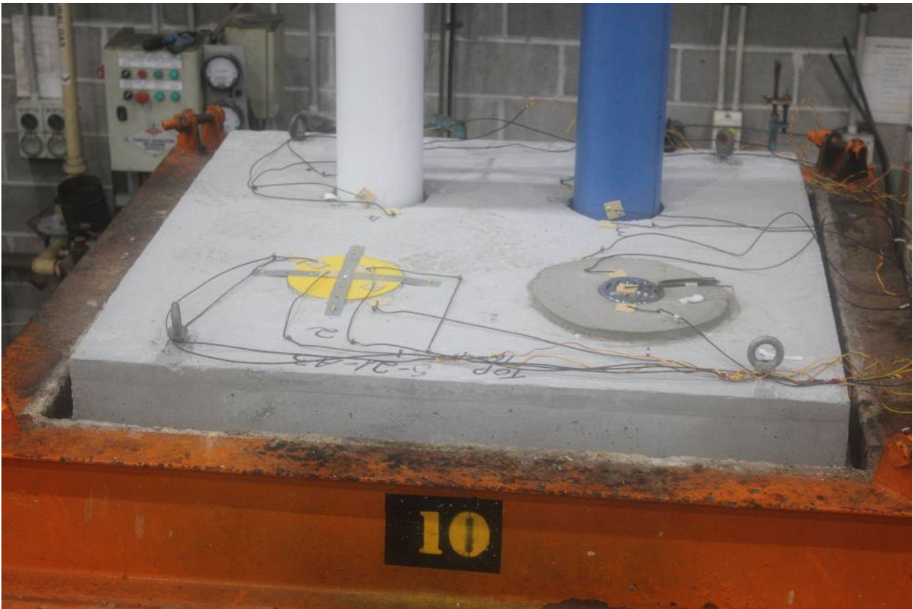
PHOTOGRAPH 3 – UNEXPOSED FACE OF SPECIMENS PRIOR TO TESTING
