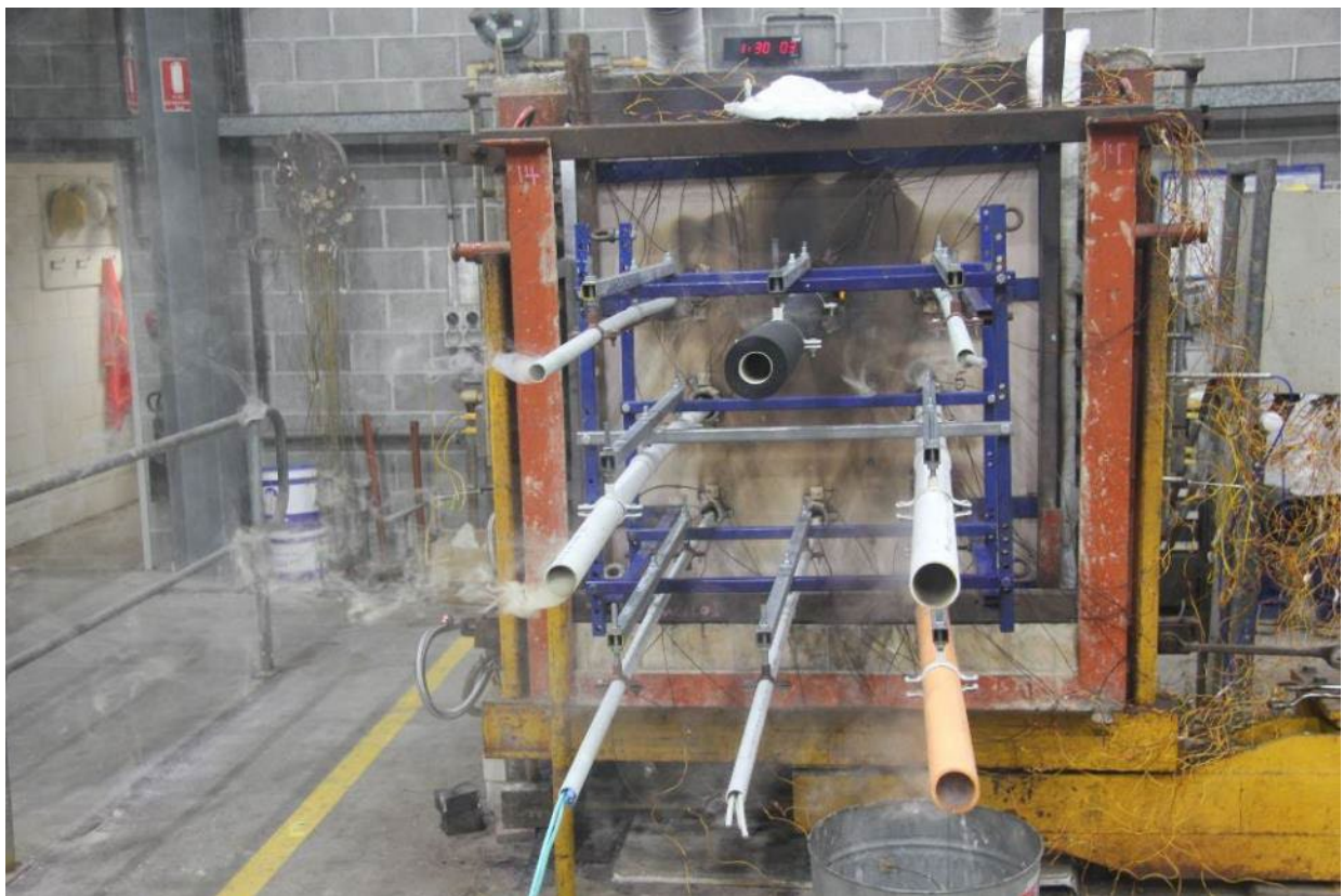
PHOTOGRAPH 10 – SPECIMENS AFTER 90 MINUTES OF TESTING
