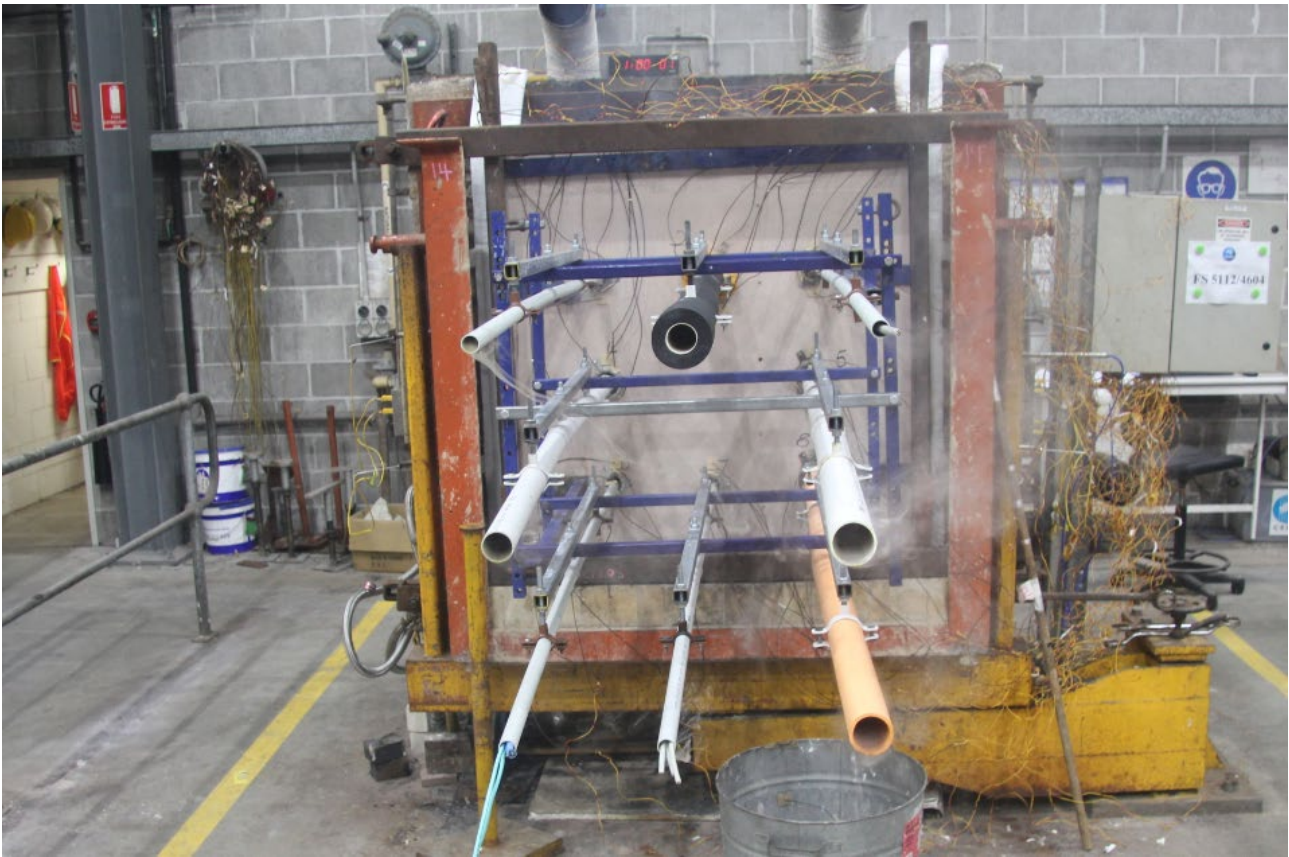
PHOTOGRAPH 7 – SPECIMENS AFTER 60 MINUTES OF TESTING
