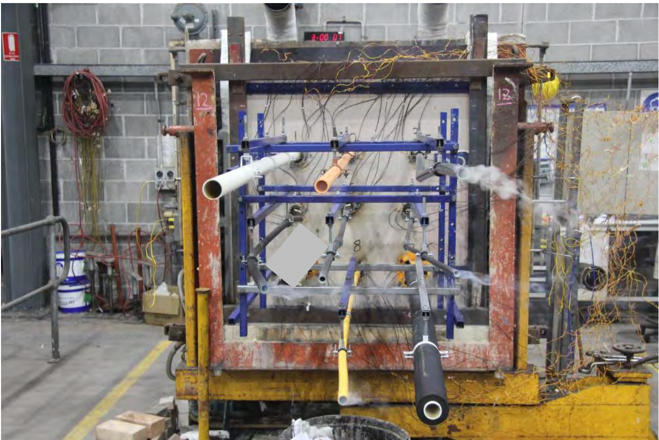
PHOTOGRAPH 10 – SPECIMENS AFTER 180 MINUTES OF TESTING
