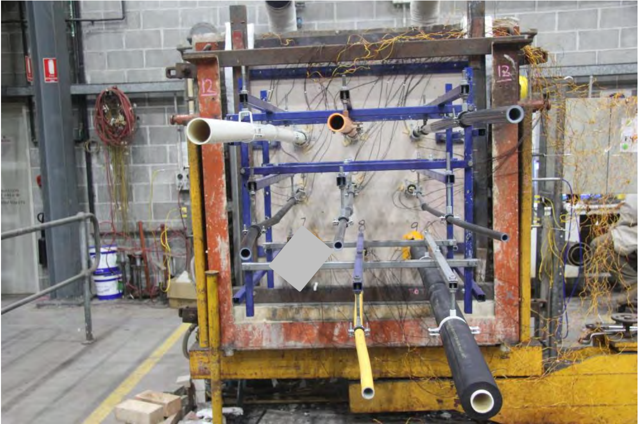
PHOTOGRAPH 6 – SPECIMENS AFTER 60 MINUTES OF TESTING
