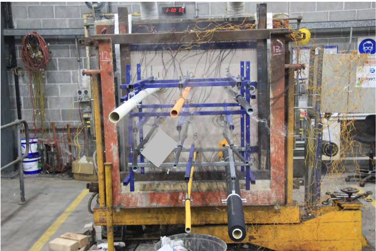
PHOTOGRAPH 8 – SPECIMENS AFTER 120 MINUTES OF TESTING
