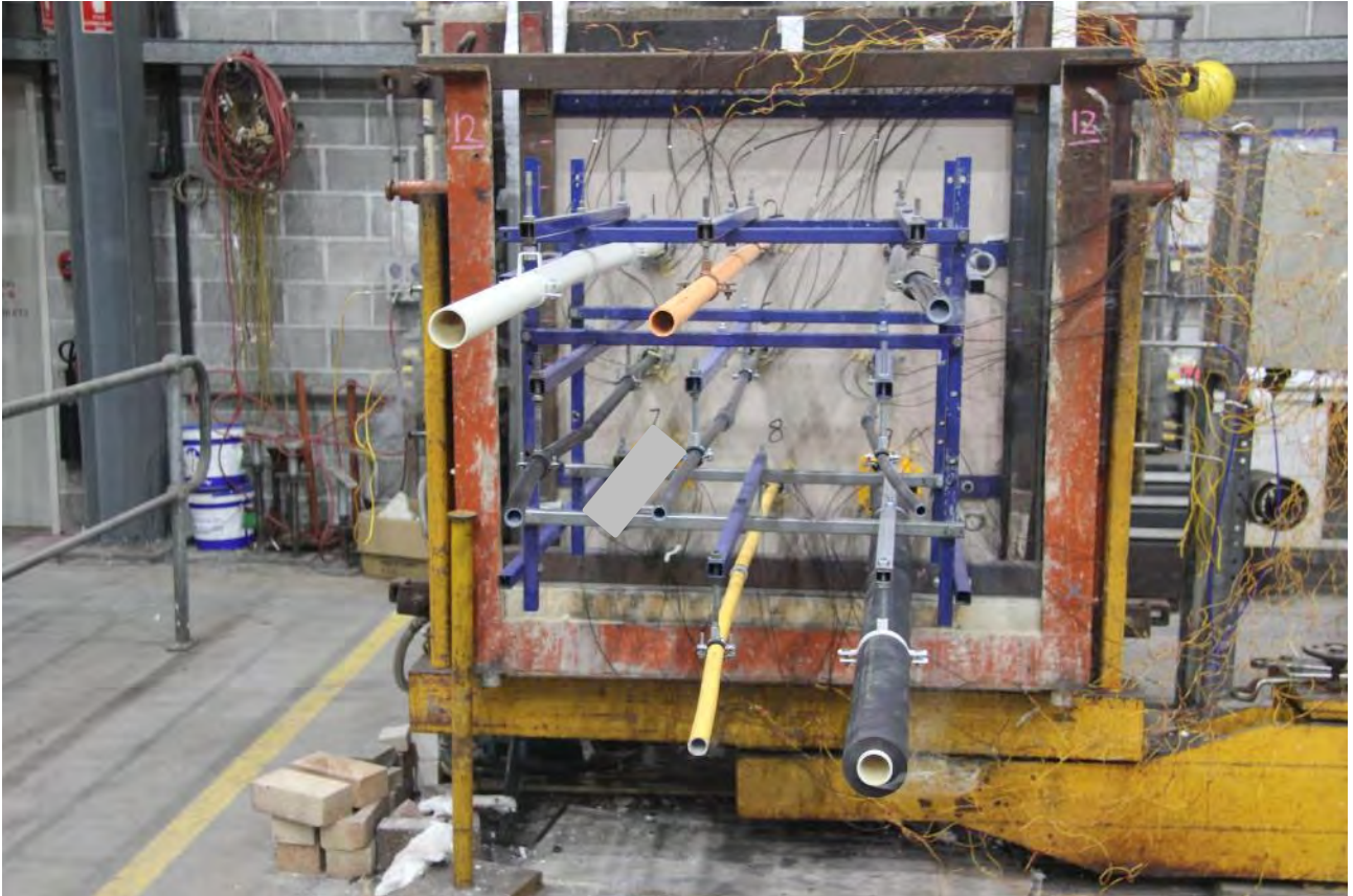
PHOTOGRAPH 4 – SPECIMENS AFTER 5 MINUTES OF TESTING
