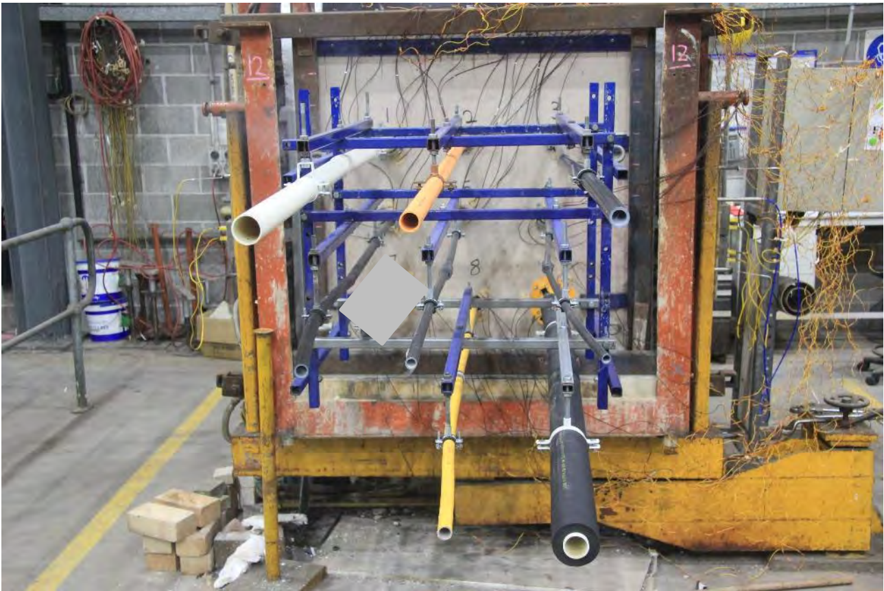
PHOTOGRAPH 7 – SPECIMENS AFTER 90 MINUTES OF TESTING
