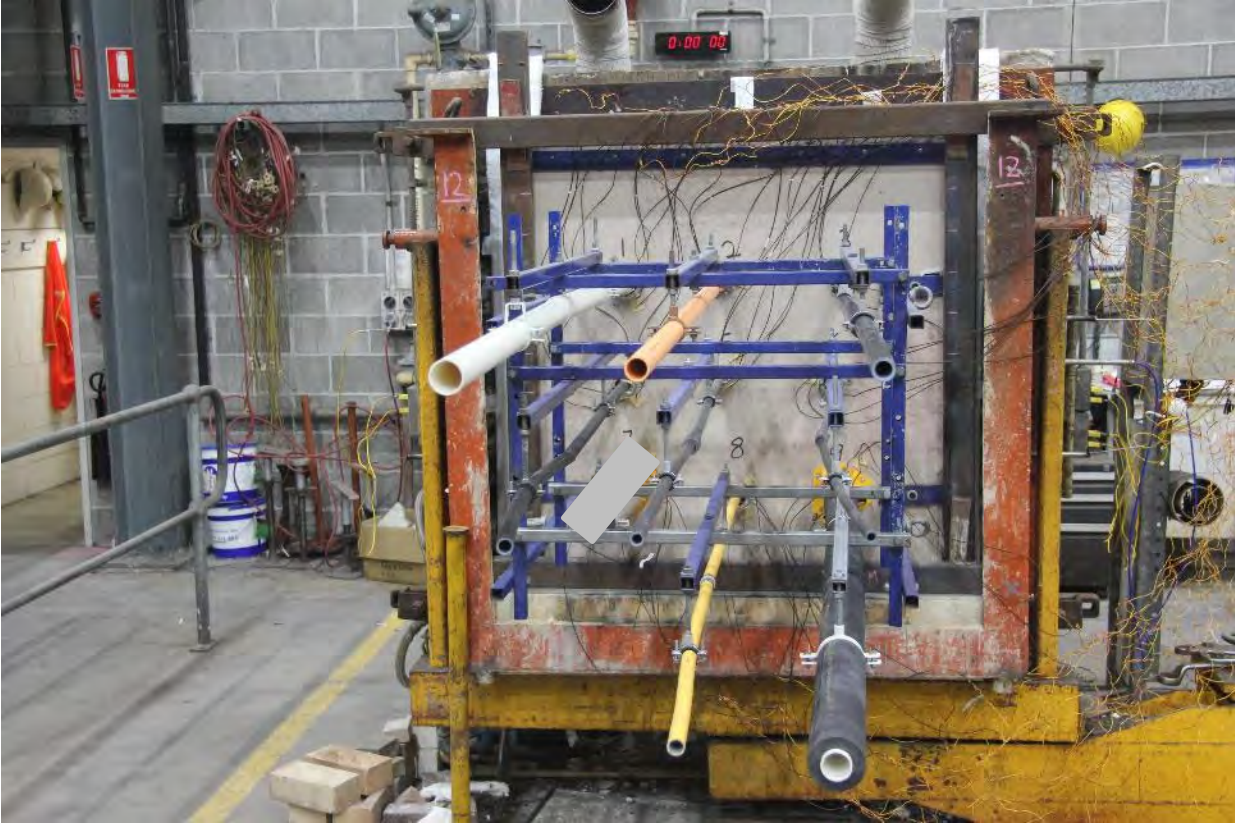
PHOTOGRAPH 1 – UNEXPOSED FACE OF SPECIMENS PRIOR TO TESTING
