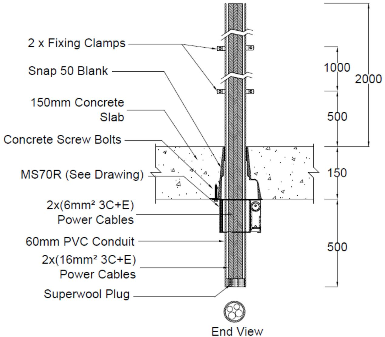
**DRAWING TITLED 'SPECIMEN #1 50 PVC CONDUIT WITH 16MM<sup>2</sup> 3C+E & 6MM<sup>2</sup> 3C+E POWER CABLES & MS70R', DATED 28 JULY 2020, PROVIDED BY SNAP FIRE SYSTEMS PTY LTD**
