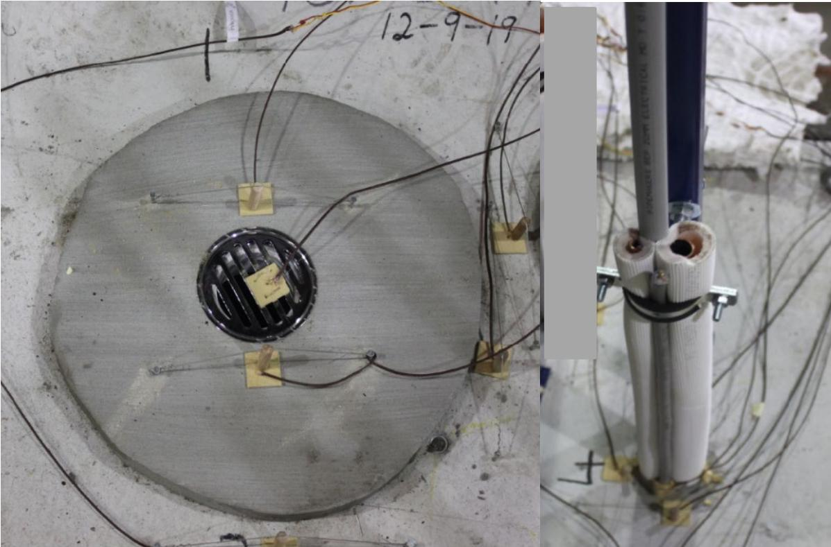
**PHOTOGRAPH 2 – UNEXPOSED FACE OF SPECIMENS 1 AND 4 PRIOR TO TESTING**
