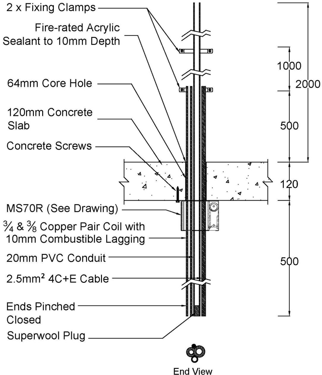
**DRAWING TITLED "SPECIMEN #4  $\frac{3}{4}$ -IN AND A  $\frac{3}{8}$ -IN INSULATED COPPER PAIR COIL, 20 PVC CONDUIT, 3 CORE CABLE + E & MS70R", DATED 12 SEPTEMBER 2019, PROVIDED BY SNAP FIRE SYSTEMS PTY LTD**
