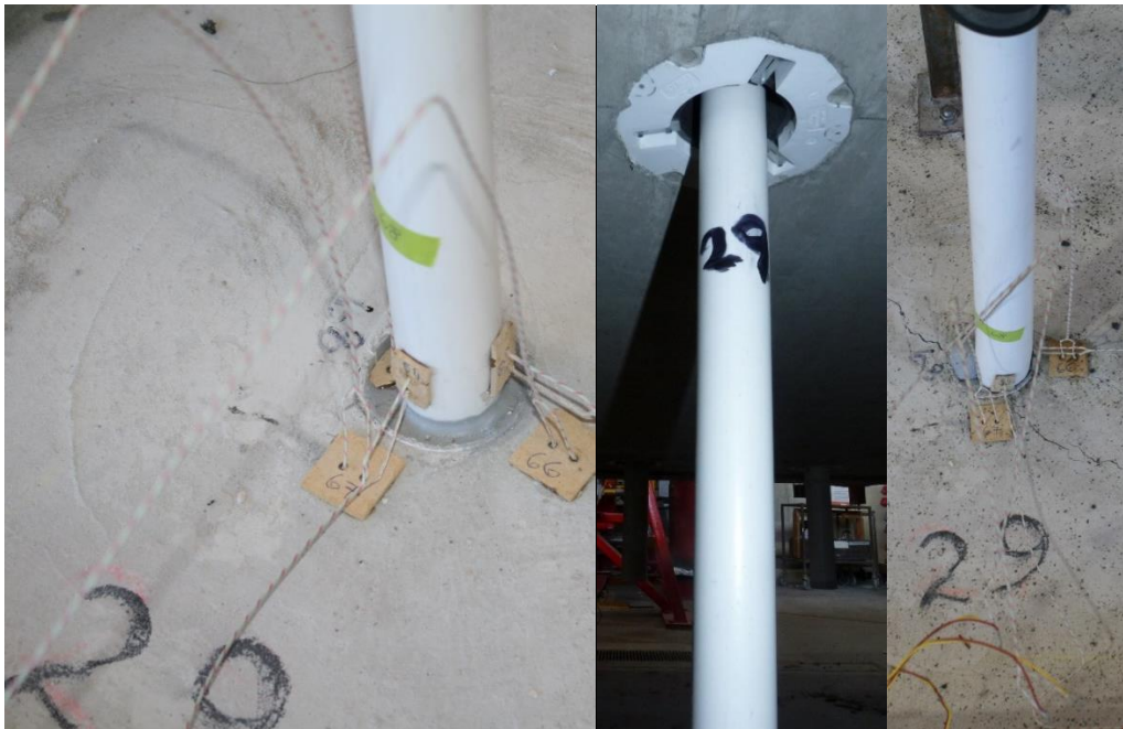
Photo 33: Specimen 29, Left to Right, Unexposed, Exposed and Unexposed Post Test
