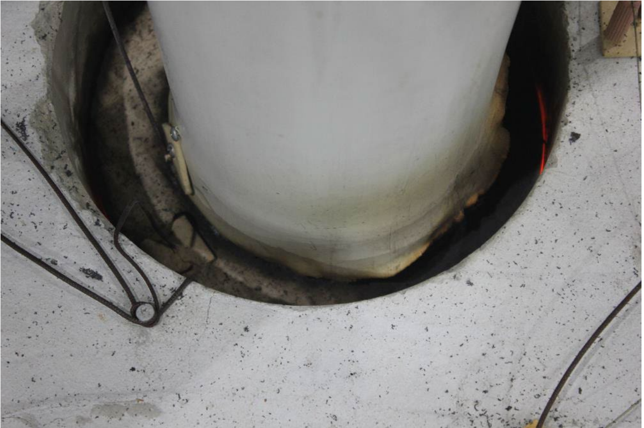
PHOTOGRAPH 15 – SPECIMEN 1 AT 240 MINUTES INTO THE TEST
