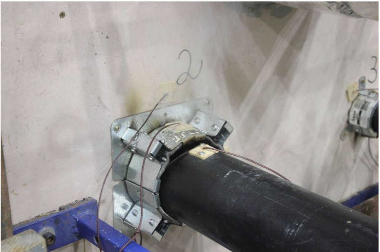
PHOTOGRAPH 12 –SPECIMEN 2 AFTER 120 MINUTES OF TESTING
