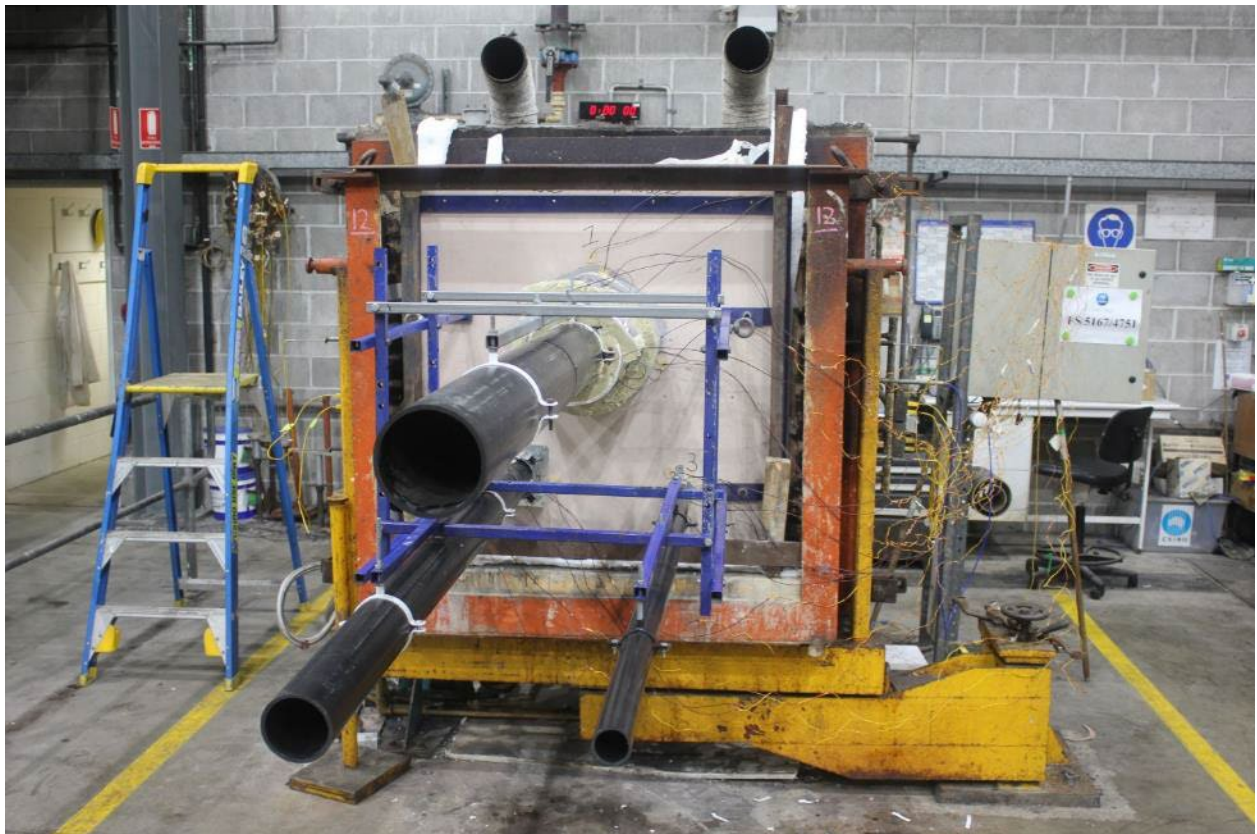
PHOTOGRAPH 2 – UNEXPOSED FACE OF SPECIMENS PRIOR TO TESTING
