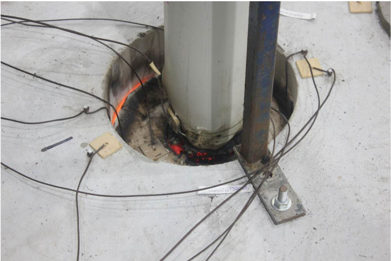
PHOTOGRAPH 17 – SPECIMEN 1 AT 181 MINUTES INTO THE TEST
