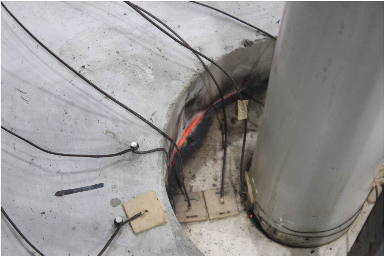
PHOTOGRAPH 15 – SPECIMEN 1 AT 160 MINUTES INTO THE TEST
