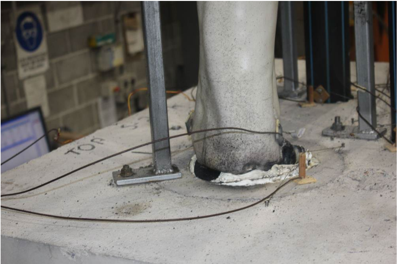
PHOTOGRAPH 14 – THE BASE OF SPECIMEN 1 AT 183 MINUTES INTO THE TEST
