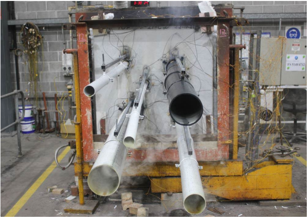
PHOTOGRAPH 17 – SPECIMENS AFTER 210 MINUTES OF TESTING
