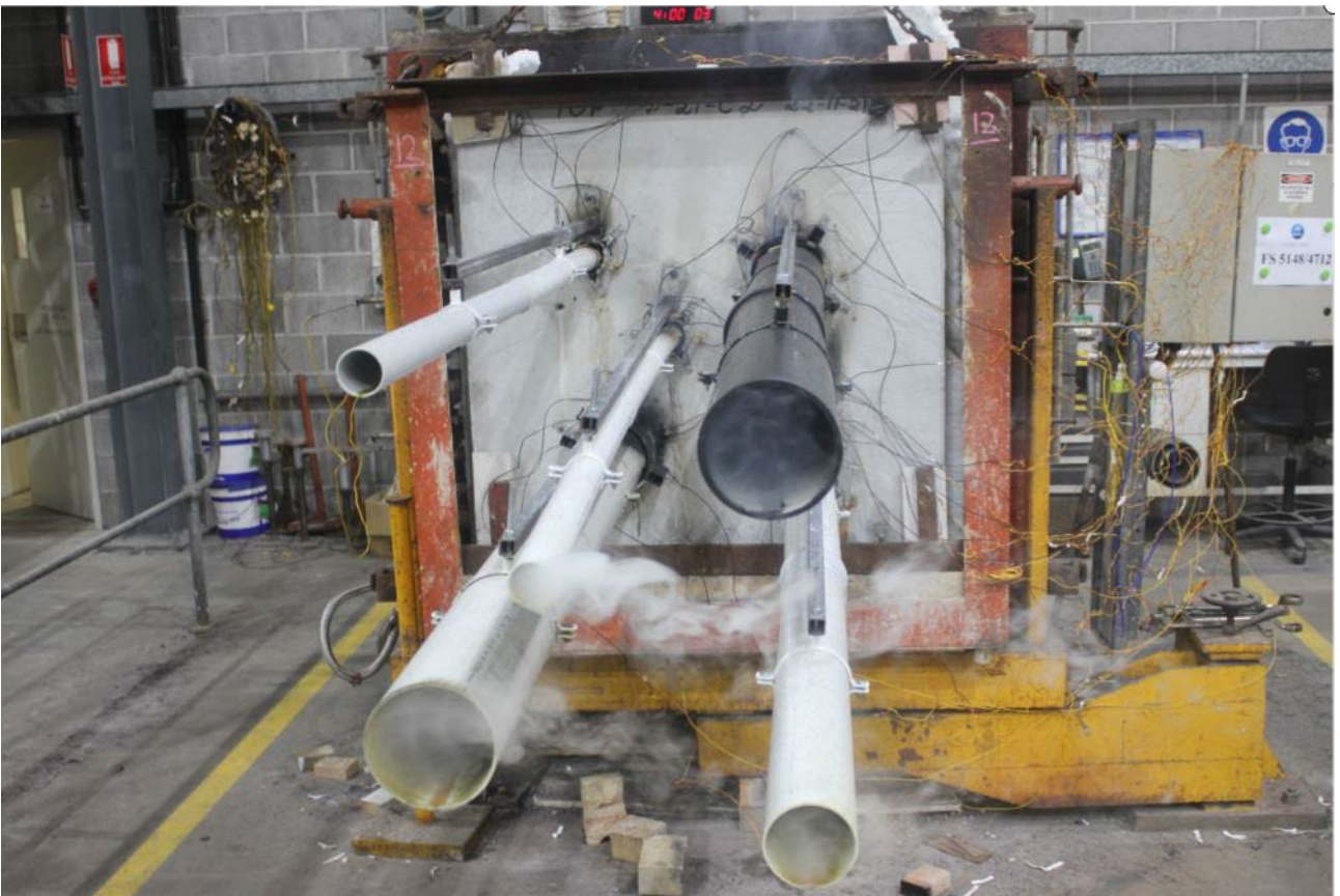
PHOTOGRAPH 20 – SPECIMENS AFTER 240 MINUTES OF TESTING
