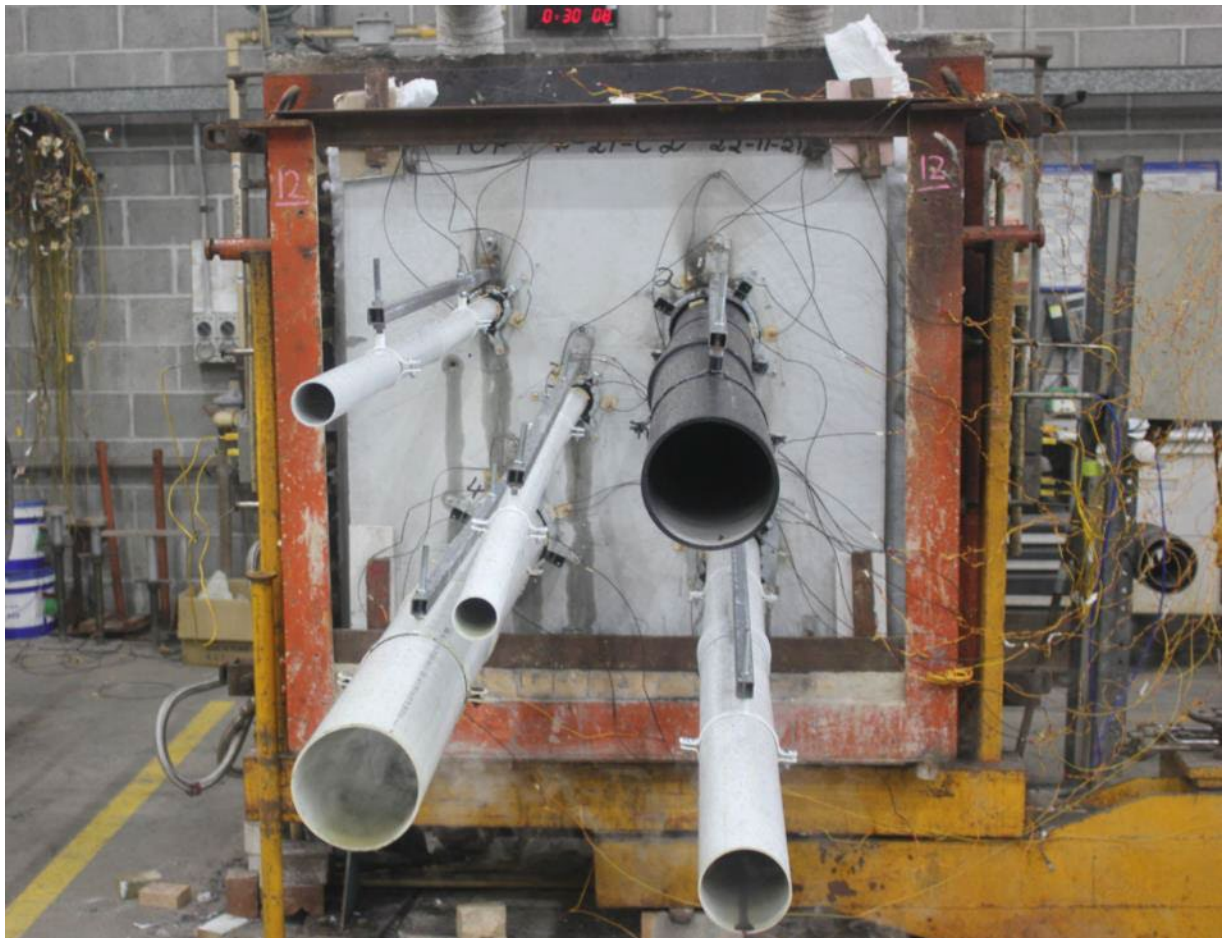
PHOTOGRAPH 6 – SPECIMENS AFTER 30 MINUTES OF TESTING
