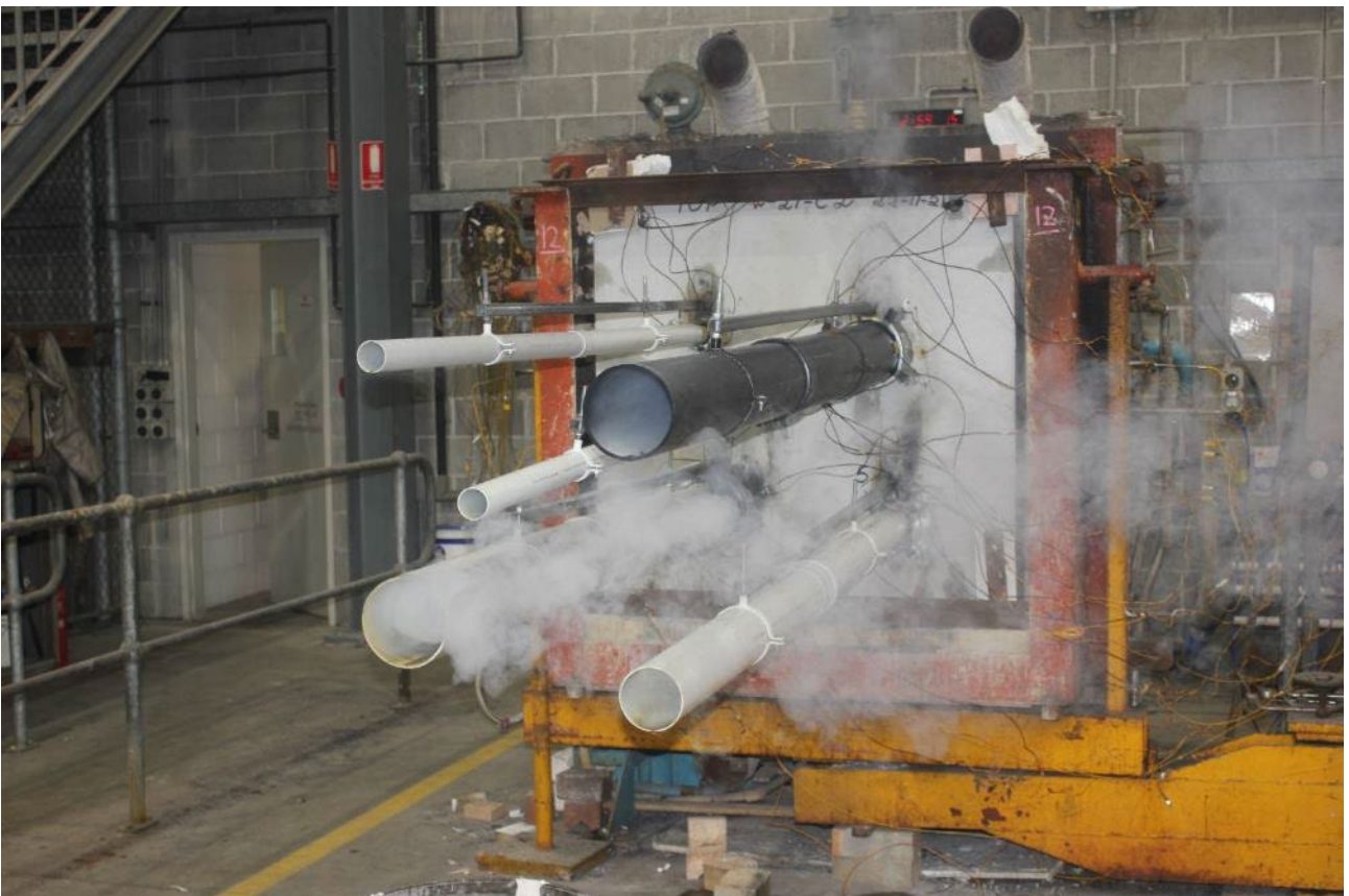
PHOTOGRAPH 14 –SPECIMENS AFTER 180 MINUTES OF TESTING
