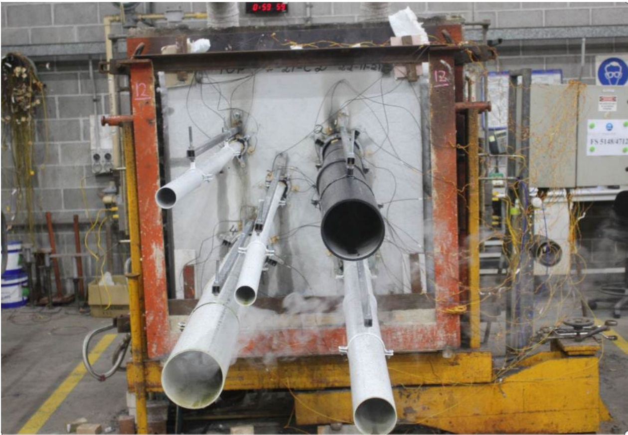
PHOTOGRAPH 7 – SPECIMENS AFTER 60 MINUTES OF TESTING
