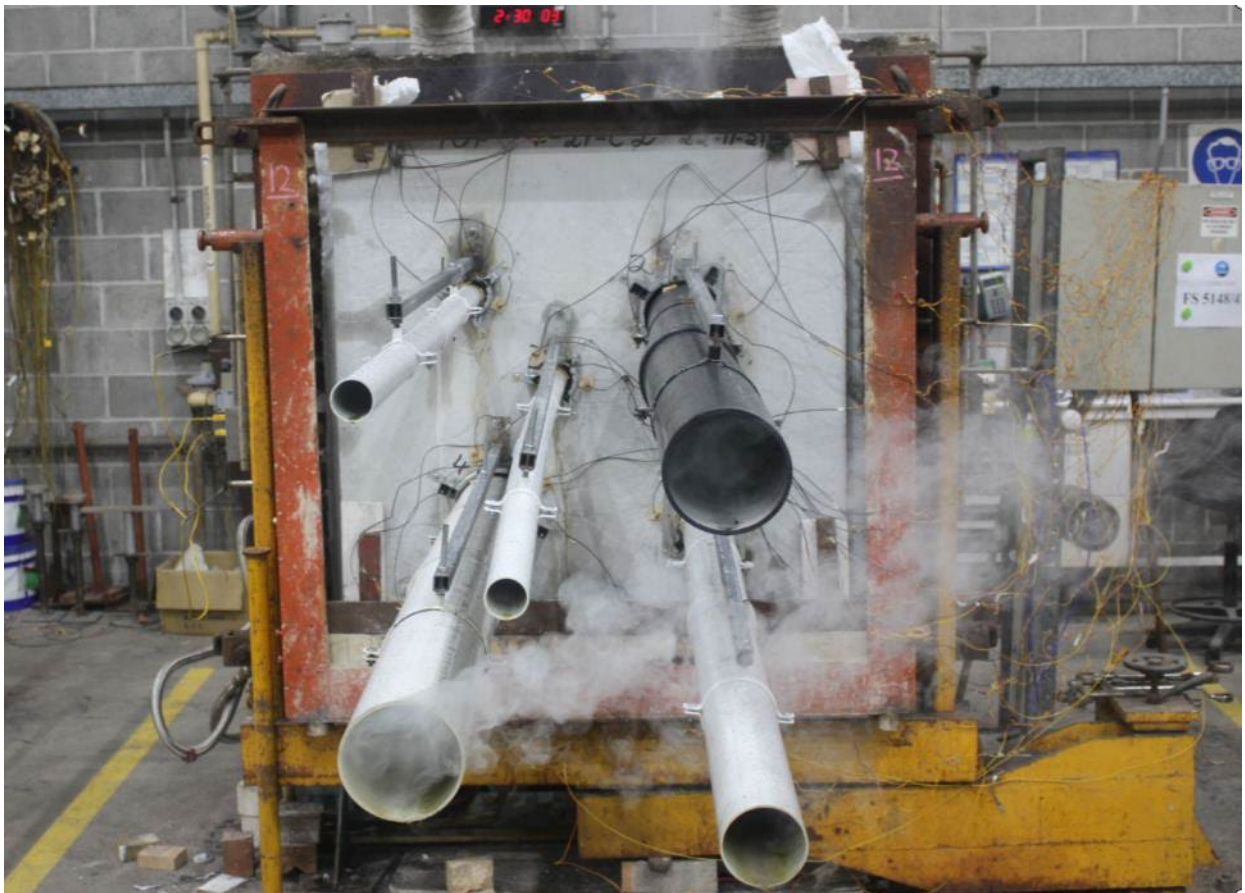
PHOTOGRAPH 10 – SPECIMENS AFTER 150 MINUTES OF TESTING
