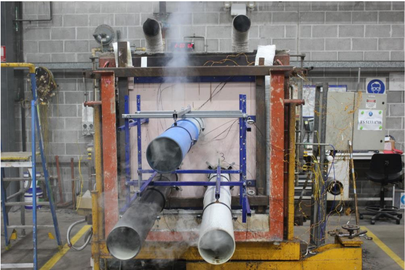
PHOTOGRAPH 13 –SPECIMENS AFTER 120 MINUTES OF TESTING
