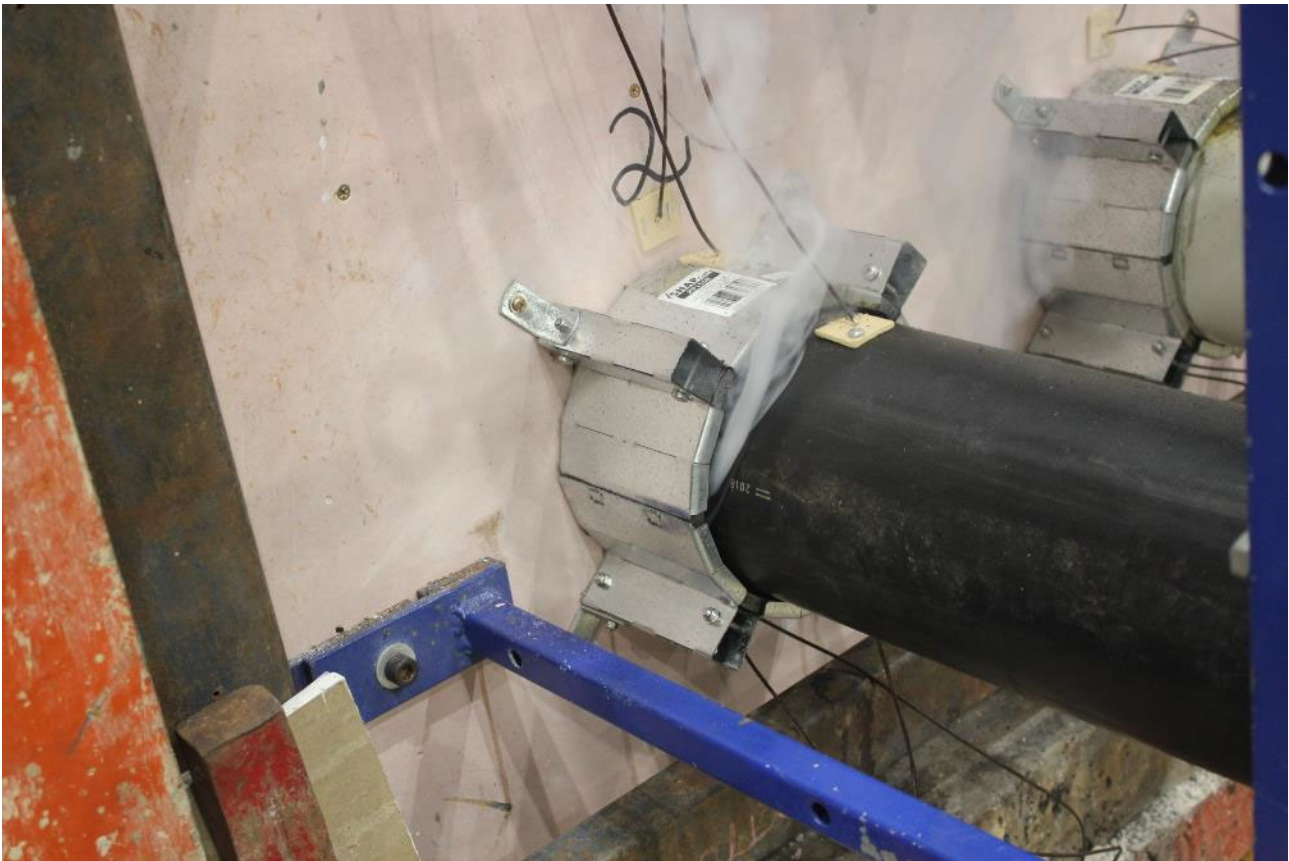
PHOTOGRAPH 9 – SPECIMEN 2 AFTER 112 MINUTES OF TESTING
