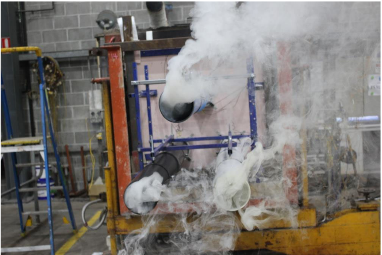
PHOTOGRAPH 4 – SPECIMENS AFTER 6 MINUTES OF TESTING
