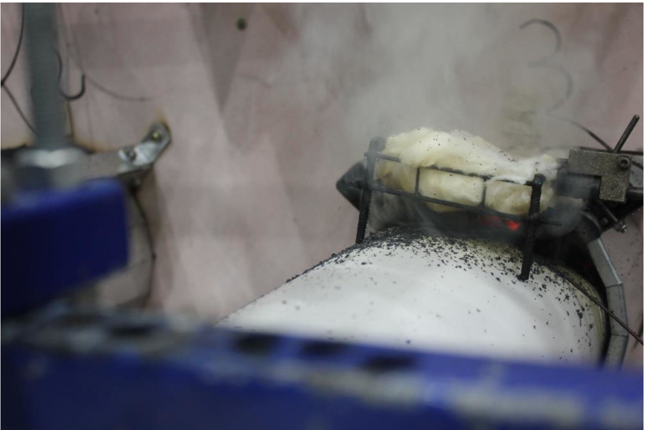
PHOTOGRAPH 16 – COTON PAD TEST APPLIED TO SPECIMEN 3 AFTER 136 MINUTES OF TESTING
