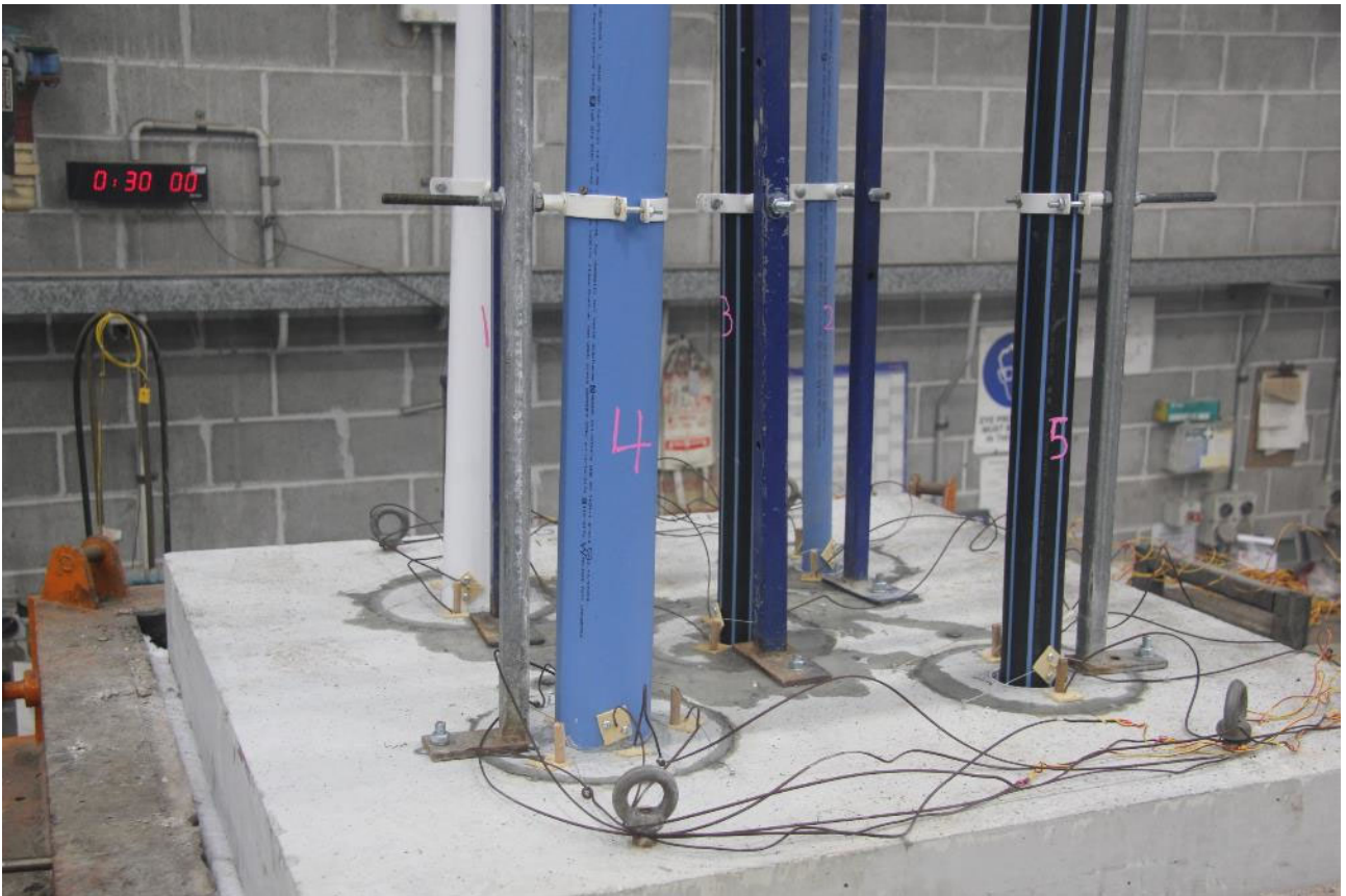
PHOTOGRAPH 5 – UNEXPOSED FACE OF SPECIMENS AT 30 MINUTES INTO THE TEST
