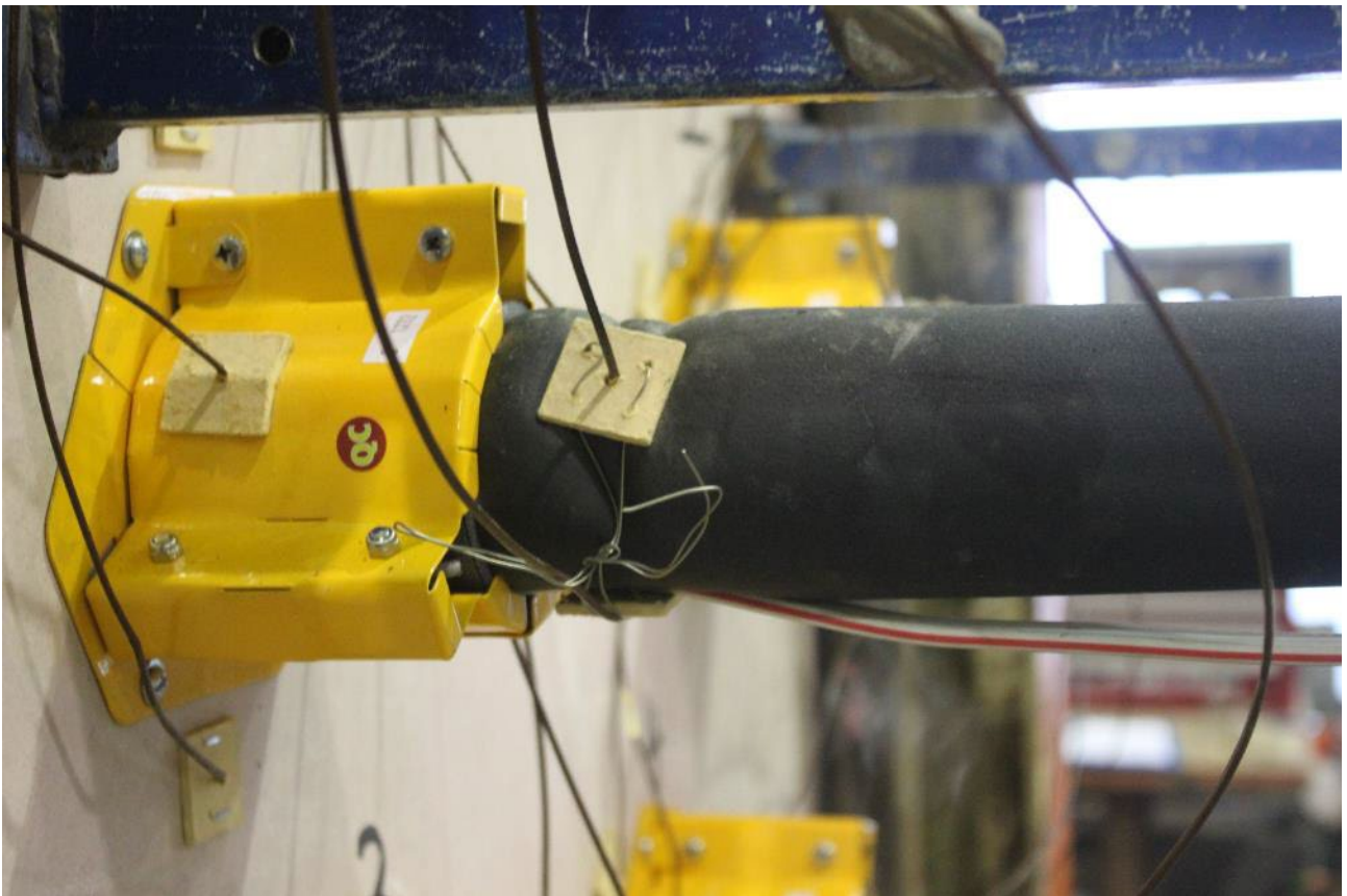
PHOTOGRAPH 5 – SPECIMEN 1 AFTER 18 MINUTES OF TESTING
