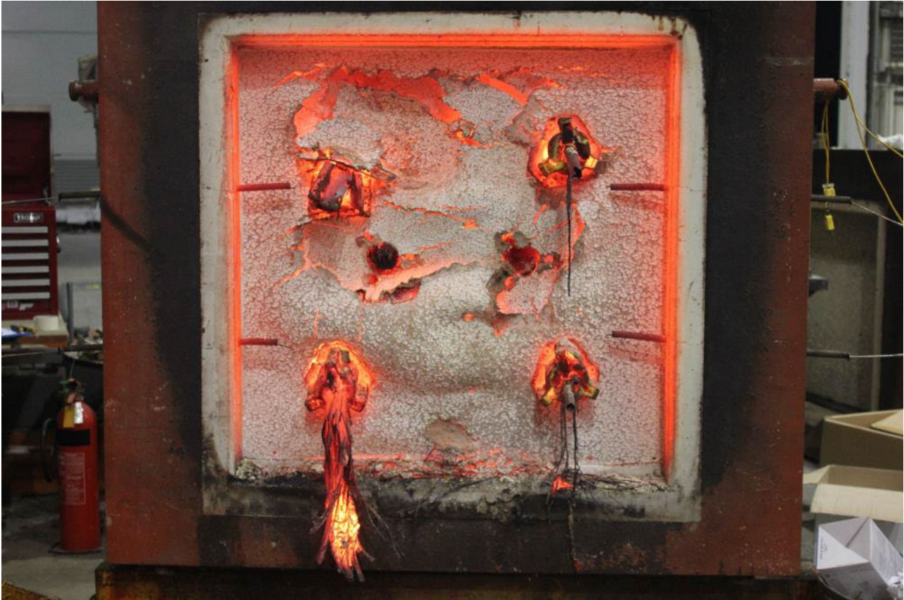
PHOTOGRAPH 16 – EXPOSED FACE OF SPECIMENS AT CONCLUSION OF TESTING
