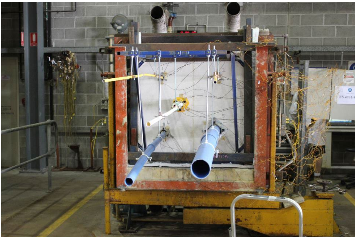
PHOTOGRAPH 2 – UNEXPOSED FACE OF SPECIMENS PRIOR TO TESTING
