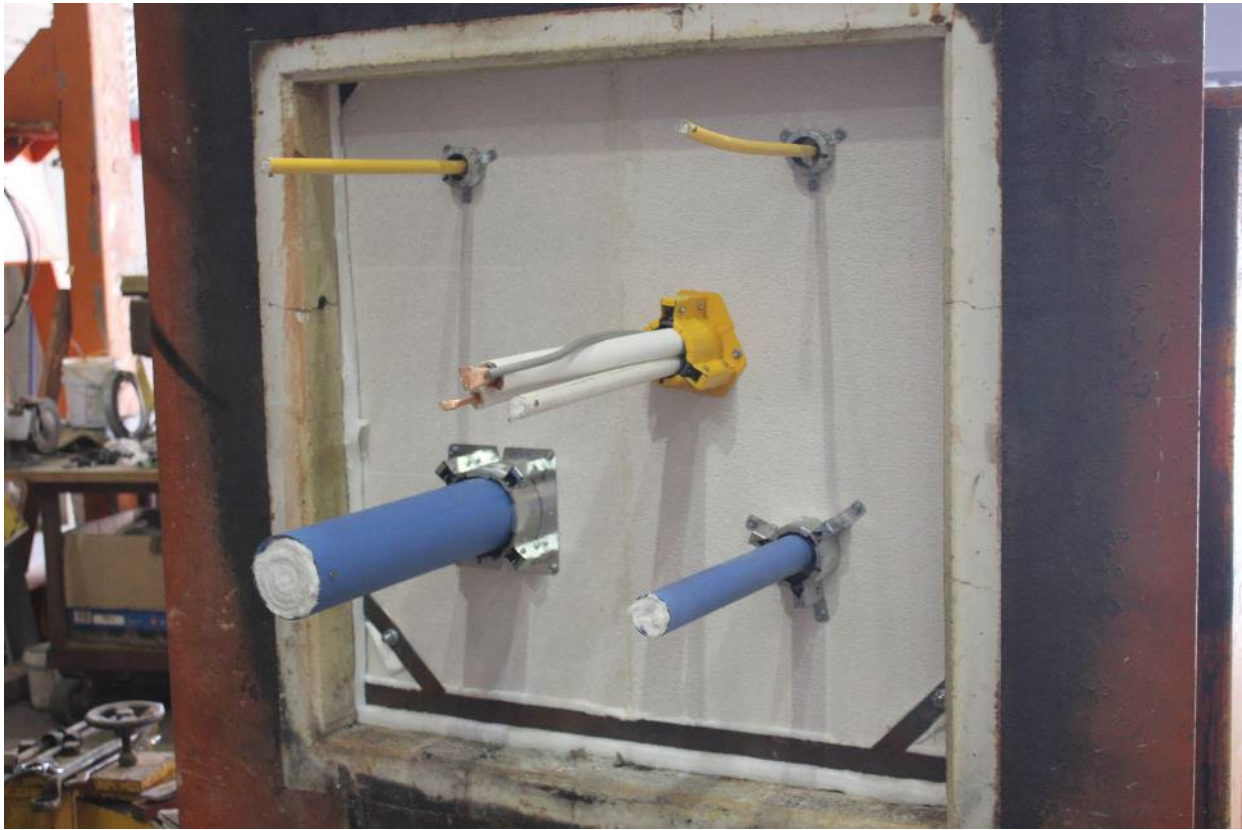
PHOTOGRAPH 1 – EXPOSED FACE OF SPECIMENS PRIOR TO TESTING
