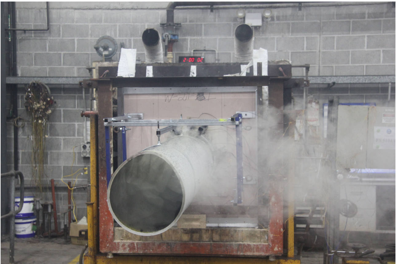
PHOTOGRAPH 12 – SPECIMEN AFTER 120 MINUTES OF TESTING
