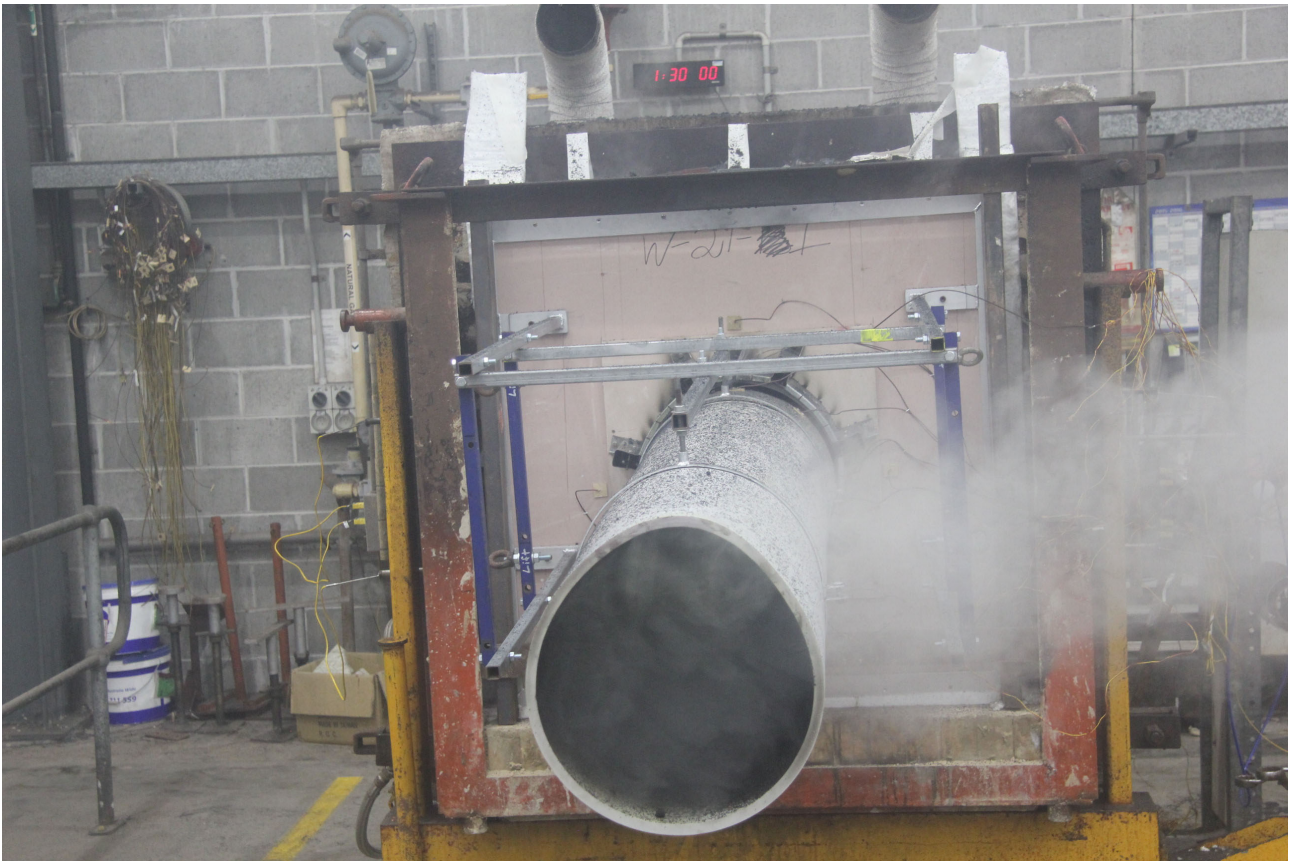
PHOTOGRAPH 11 – SPECIMENS AFTER 90 MINUTES OF TESTING
