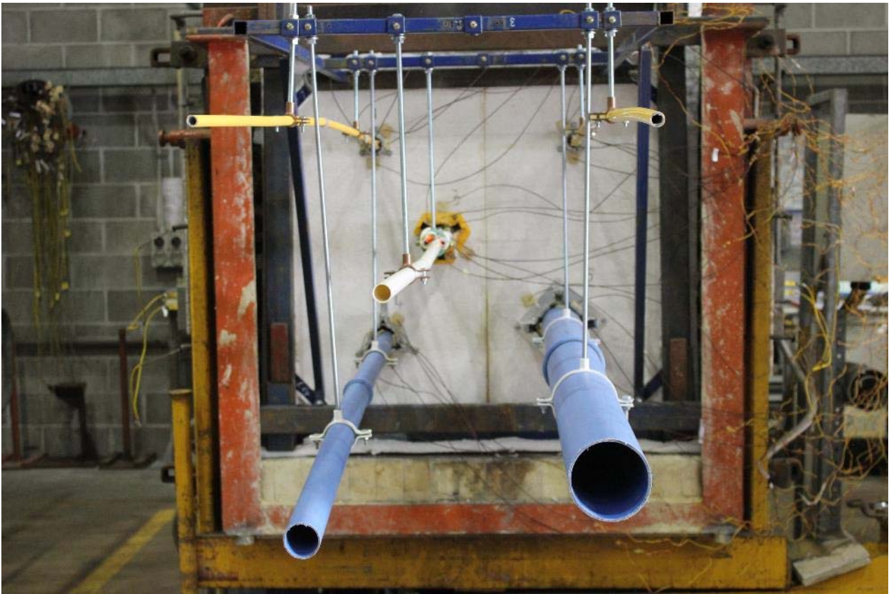
PHOTOGRAPH 7 – SPECIMENS AFTER 60 MINUTES OF TESTING
