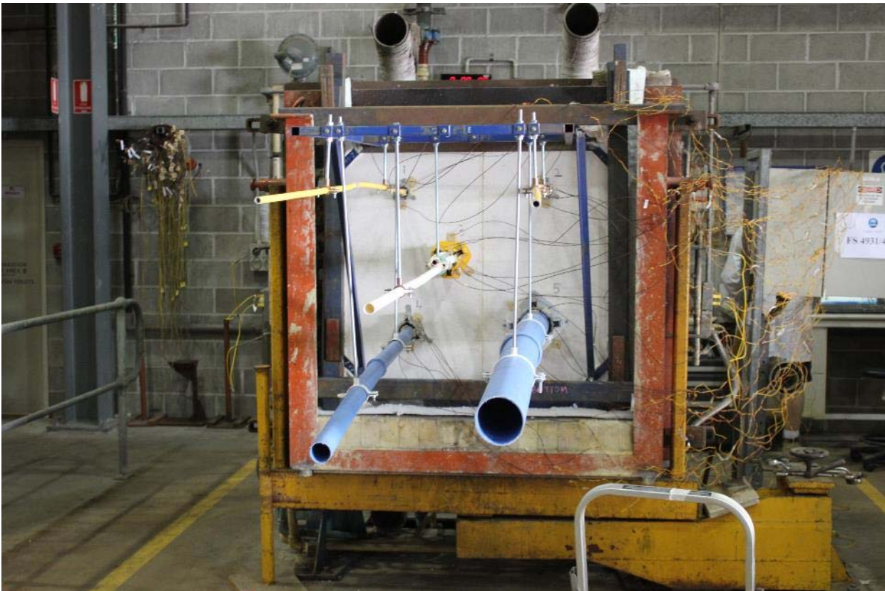
PHOTOGRAPH 2 – UNEXPOSED FACE OF SPECIMENS PRIOR TO TESTING
