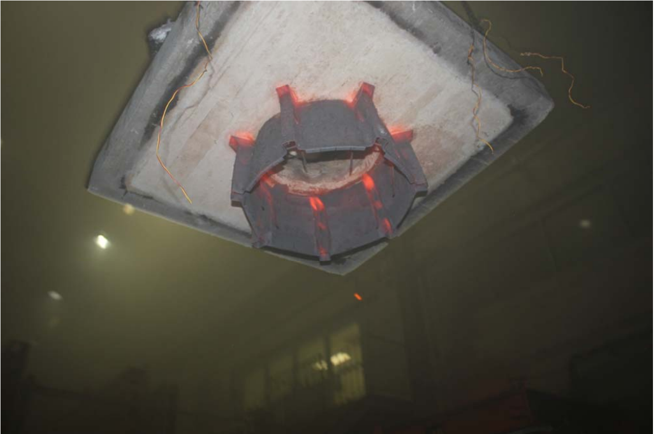
PHOTOGRAPH 14 – EXPOSED FACE OF SPECIMEN AT THE CONCLUSION OF TESTING
