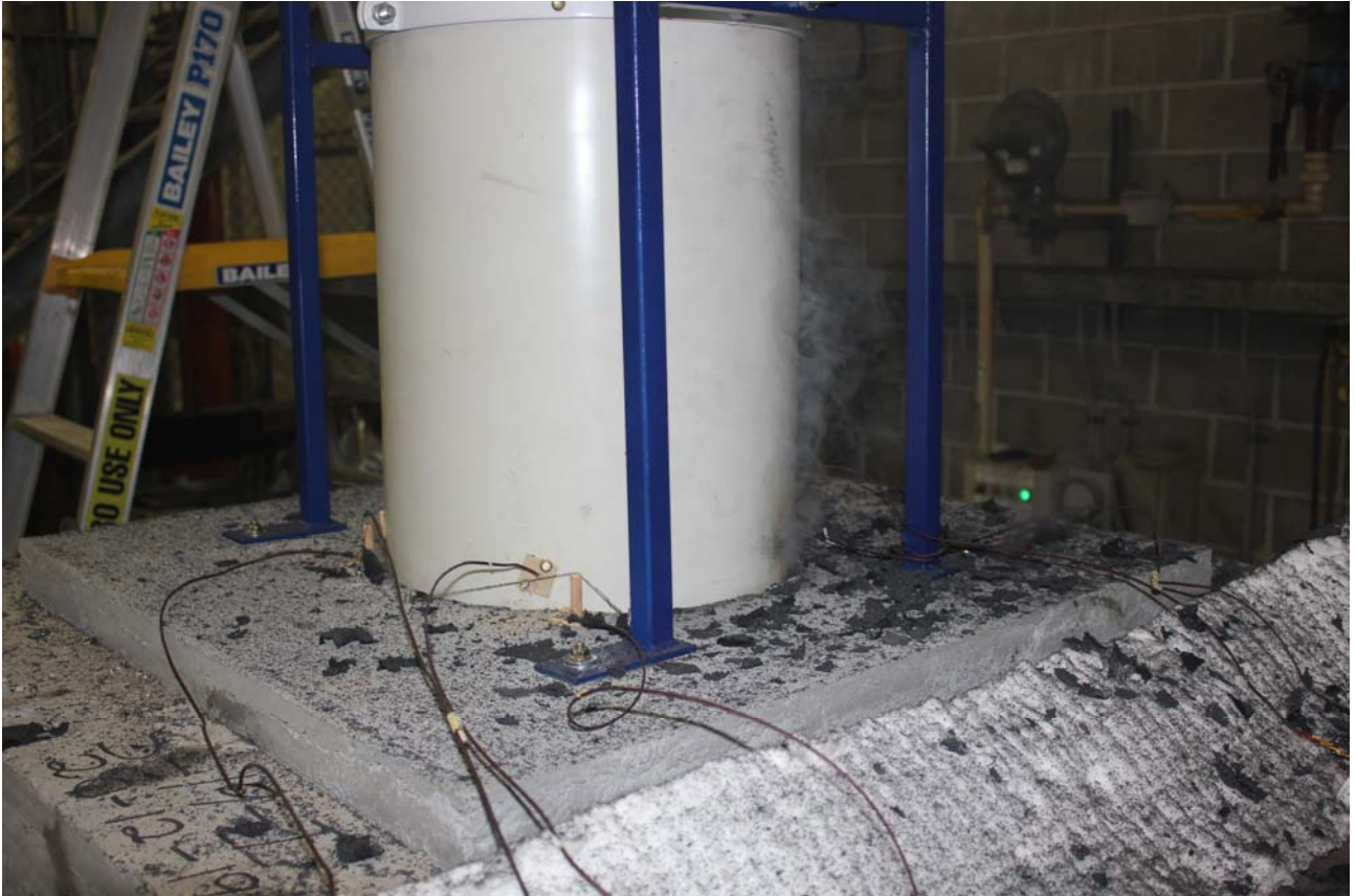
PHOTOGRAPH 10 – SPECIMEN AFTER 155MINUTES OF TESTING
