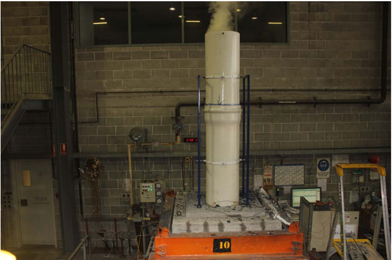
PHOTOGRAPH 8 – SPECIMEN AFTER 120 MINUTES OF TESTING
