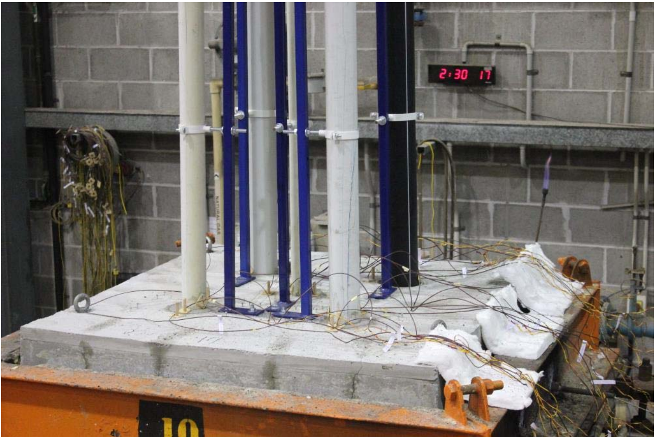
PHOTOGRAPH 7 – SPECIMENS AFTER 150 MINUTES OF TESTING
