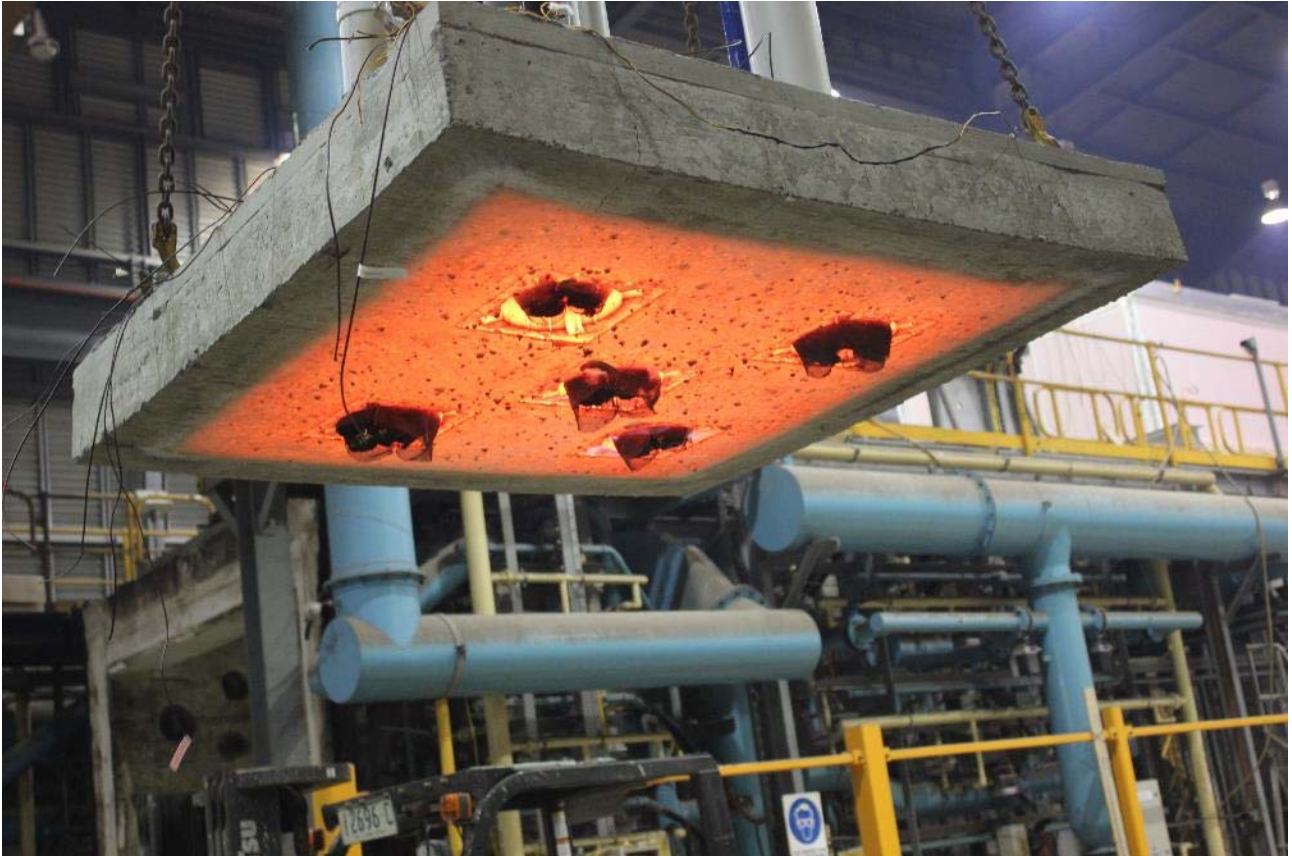
PHOTOGRAPH 12 – EXPOSED FACE OF SPECIMENS AFTER THE CONCLUSION OF TESTING
