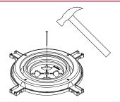
Inspect the collar to make sure it has not been damaged in transit and all components are present. Clip the collar onto the locator plate, ensuring the collar base flange (7) is flat on the formwork. Secure the collar to the formwork using preferred fixing points. Fit the cap (1) into the top of the collar. Generally, black collars are for Floorwaste and Shower applications. White collars are for Stackwork only.
