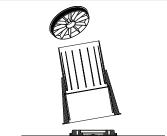
Pour concrete. Snap cast-in Fire Collars are approved for use in concrete slabs of a range of thicknesses (see website: www.snapcollars.com.au for tested systems).
