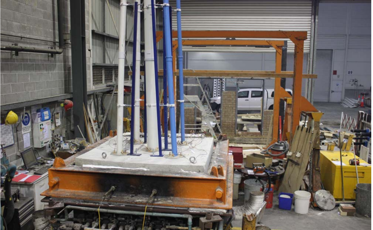
PHOTOGRAPH 11 – UNEXPOSED FACED OF SPECIMENS AT THE CONCLUSION OF TESTING
