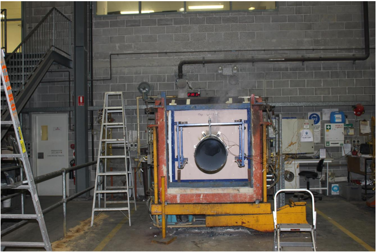
PHOTOGRAPH 9 – SPECIMEN AFTER 120 MINUTES OF TESTING
