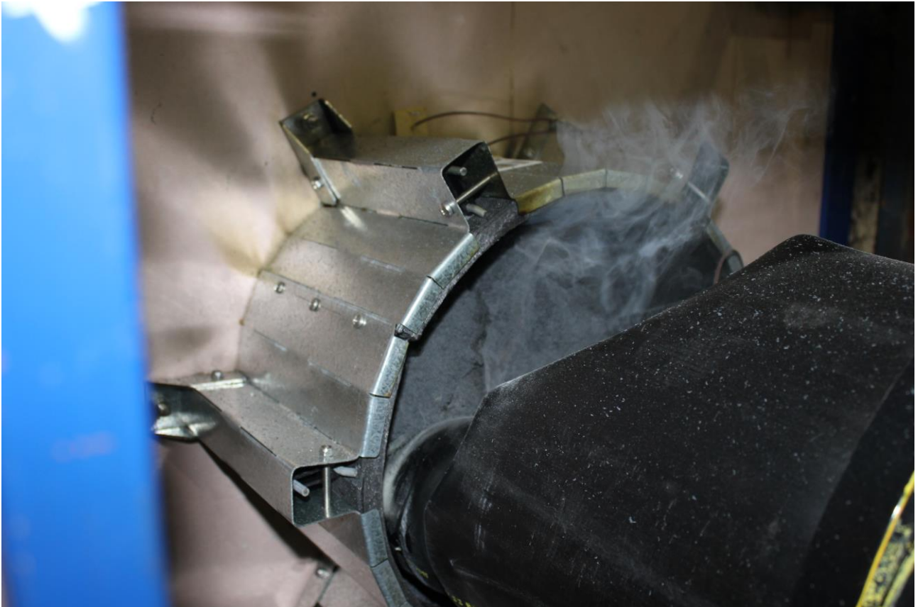
PHOTOGRAPH 10 – UNEXPOSED FACE OF SPECIMEN AT THE CONCLUSION OF TESTING
