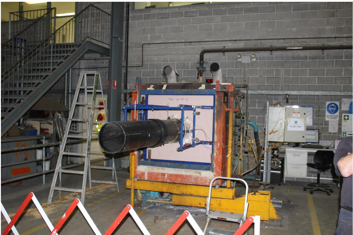
PHOTOGRAPH 2 – UNEXPOSED FACE OF SPECIMEN PRIOR TO TESTING
