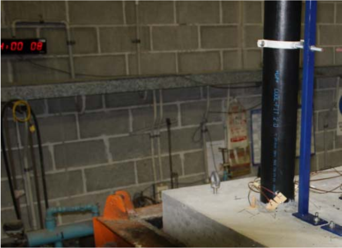
PHOTOGRAPH 7 – UNEXPOSED FACED OF SPECIMEN AT CONCLUSION OF TESTING
