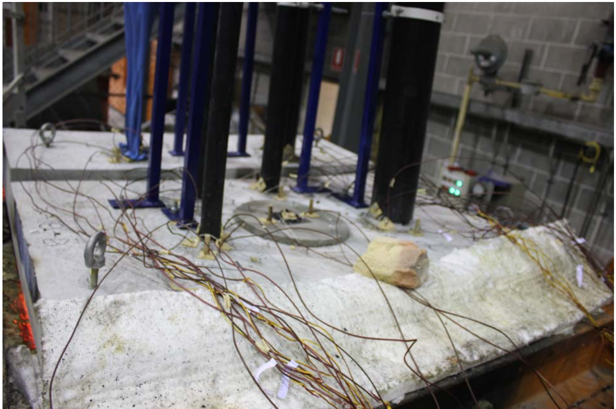
PHOTOGRAPH 5 – SPECIMENS AFTER 180 MINUTES OF TESTING
