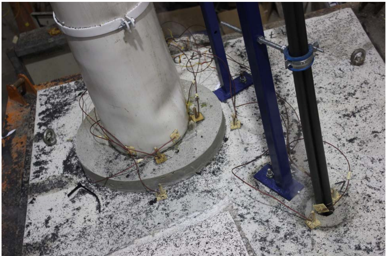
PHOTOGRAPH 6 – PENETRATIONS AFTER 120 MINUTES OF TESTING
