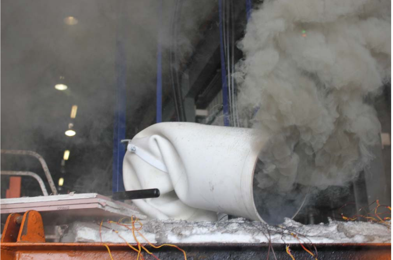
PHOTOGRAPH 3 – PENETRATION 1 AFTER 7 MINUTES OF TESTING
