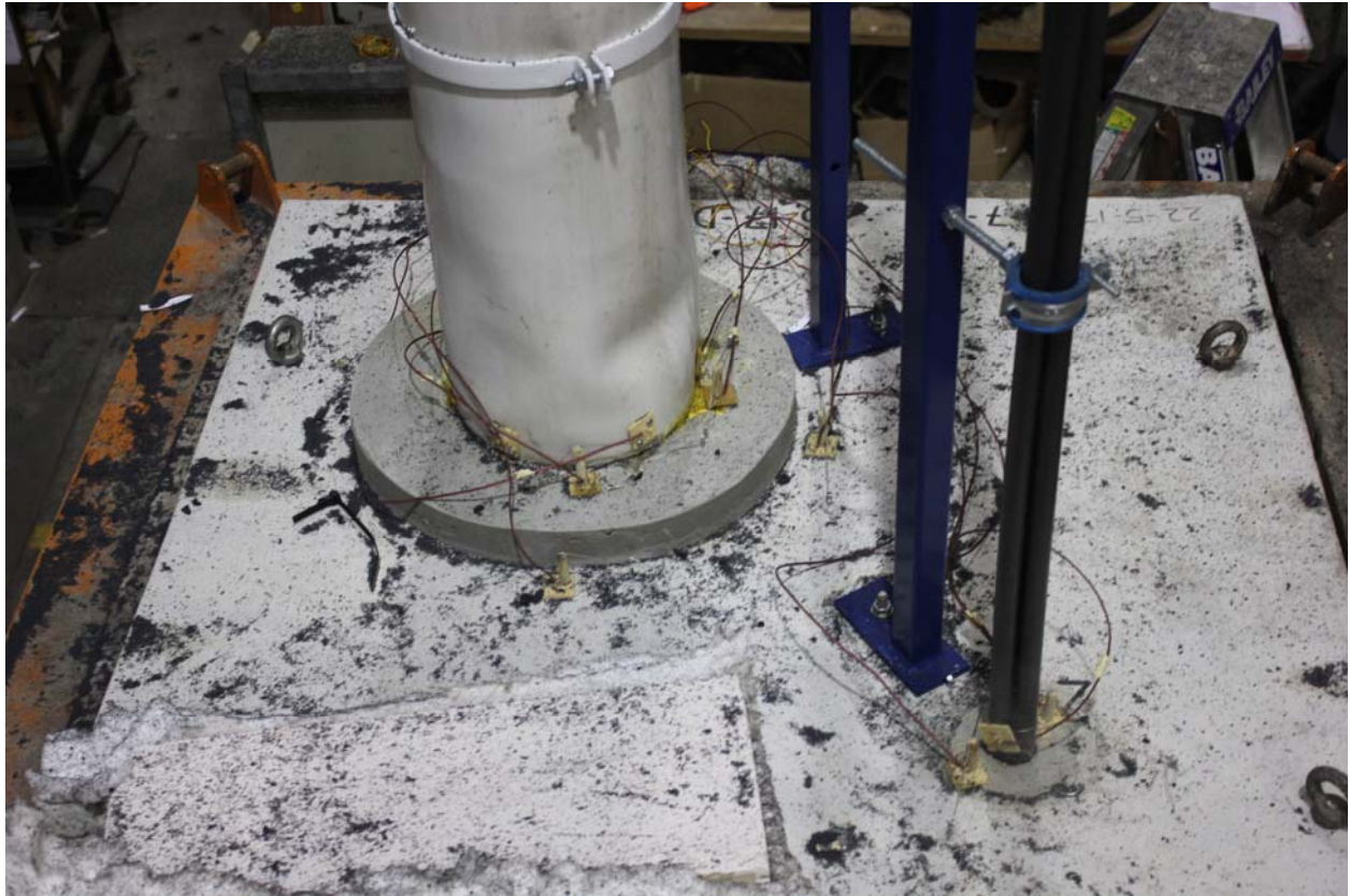
PHOTOGRAPH 7 – PENETRATIONS AFTER 180 MINUTES OF TESTING
