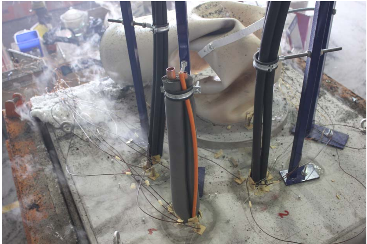
PHOTOGRAPH 5 – PENETRATIONS AFTER 60 MINUTES OF TESTING
