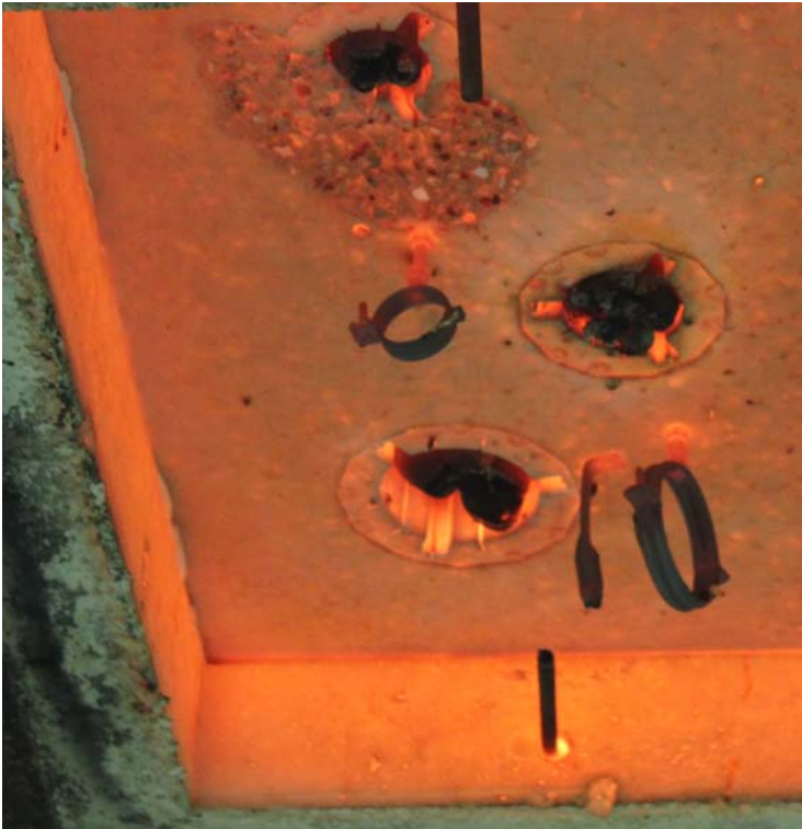
PHOTOGRAPH 6 – EXPOSED FACE OF SPECIMENS AT CONCLUSION OF TESTING
