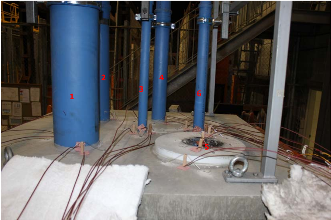
PHOTOGRAPH 2 – UNEXPOSED FACE OF SPECIMENS PRIOR TO TESTING
