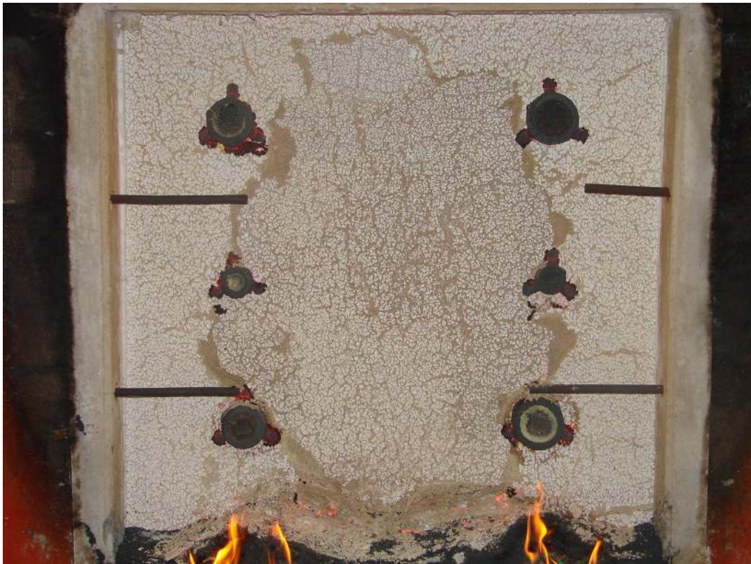
Photograph 7 – Exposed face of the specimen after the conclusion of testing
