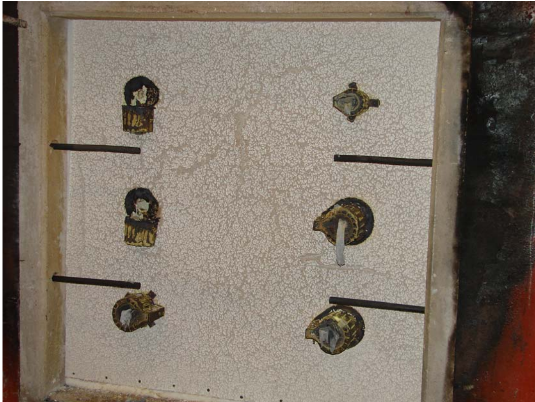
Photograph 7 – Exposed face after the conclusion of testing
