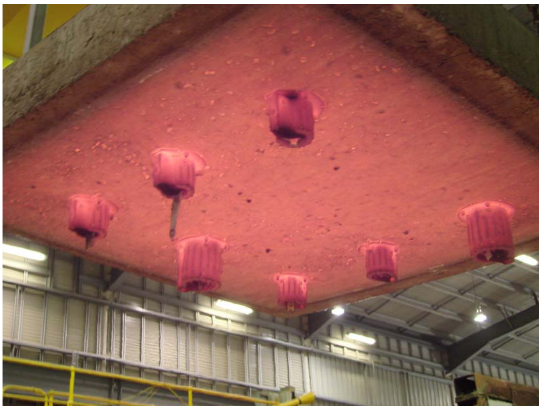
Photograph 8 – Exposed face of the specimen after the conclusion of testing
