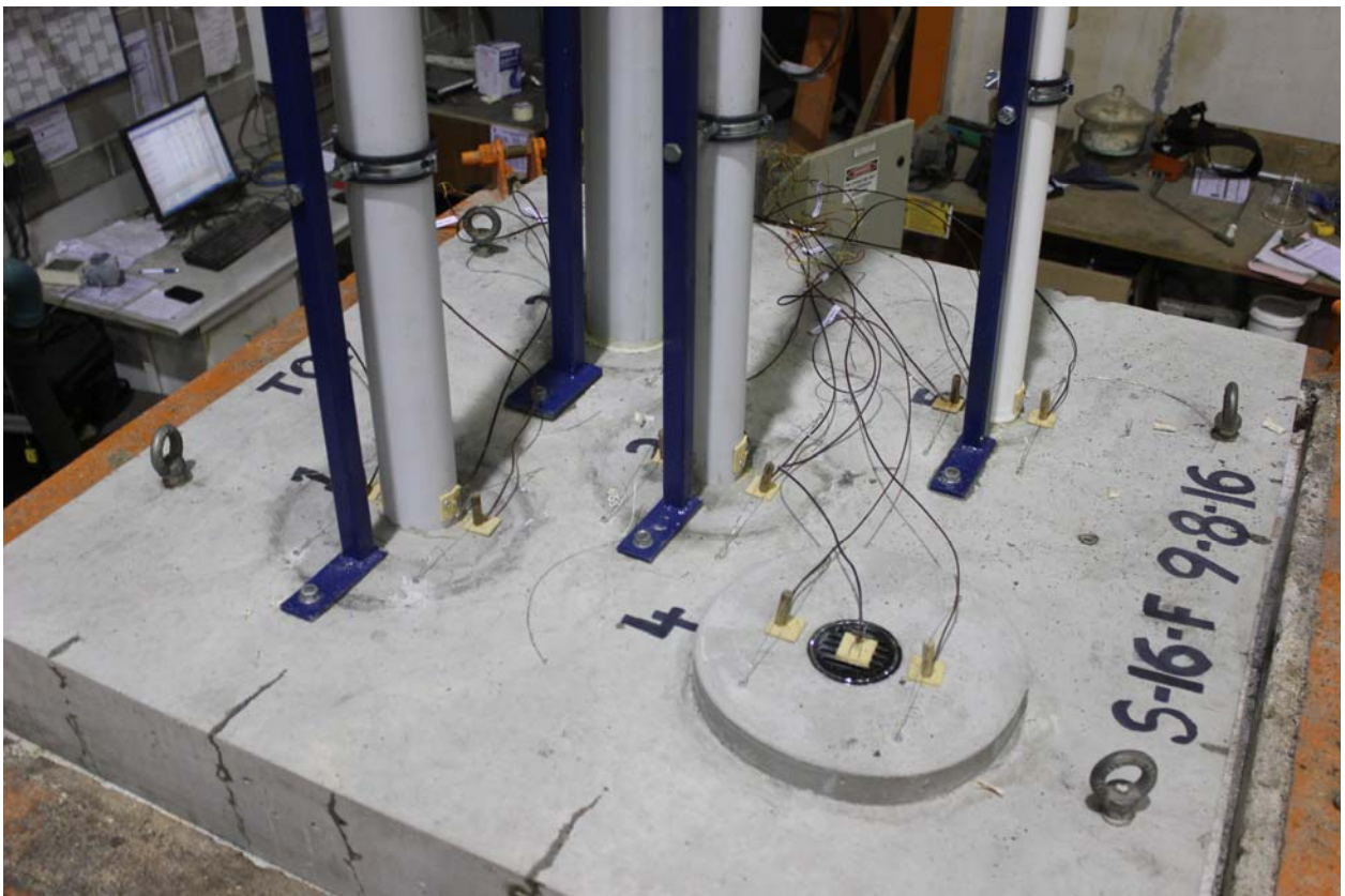
PHOTOGRAPH 4 – SPECIMENS AFTER 120 MINUTES OF TESTING
