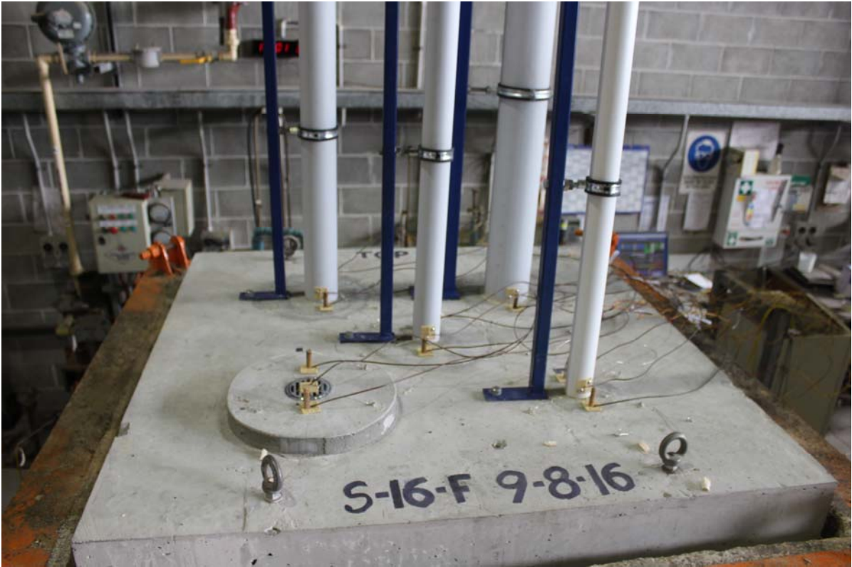
PHOTOGRAPH 2 – UNEXPOSED FACE OF SPECIMENS PRIOR TO TESTING
