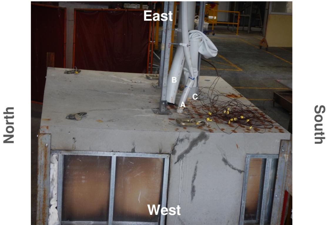
Figure 15 Unexposed face of specimen at the end of test
