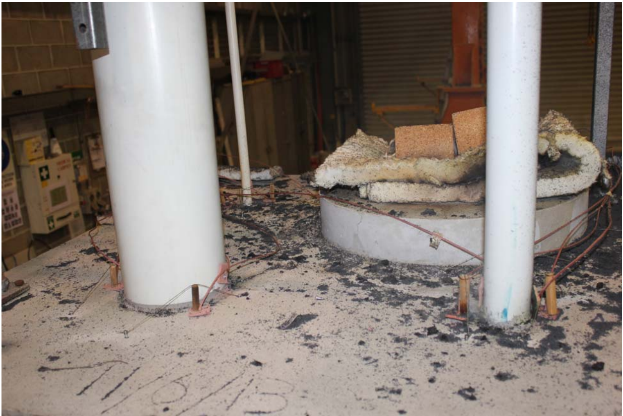
PHOTOGRAPH 5 – SPECIMENS AFTER 180 MINUTES OF TESTING
