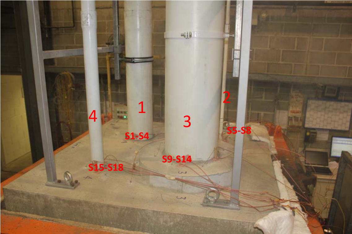
PHOTOGRAPH 2 – UNEXPOSED FACE OF SPECIMENS PRIOR TO TESTING
