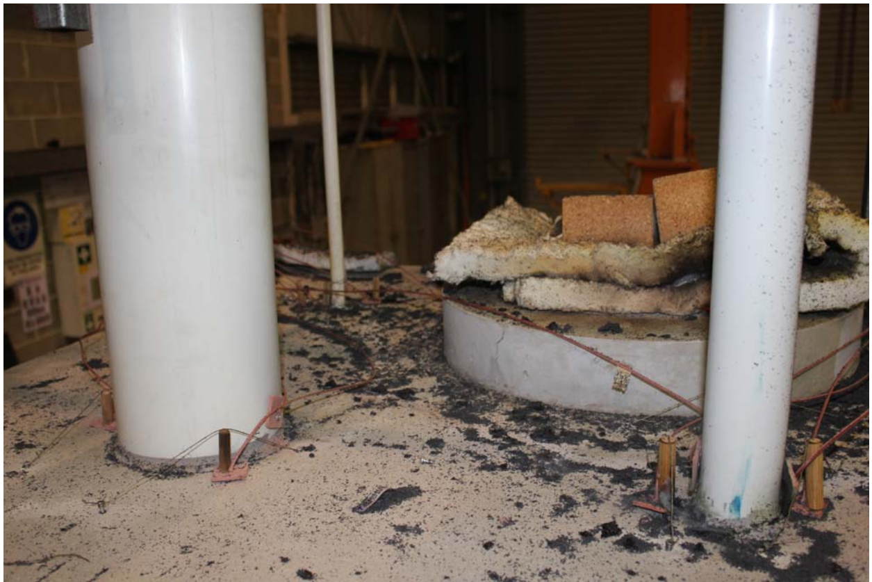
PHOTOGRAPH 6 – SPECIMENS AFTER 240 MINUTES OF TESTING
