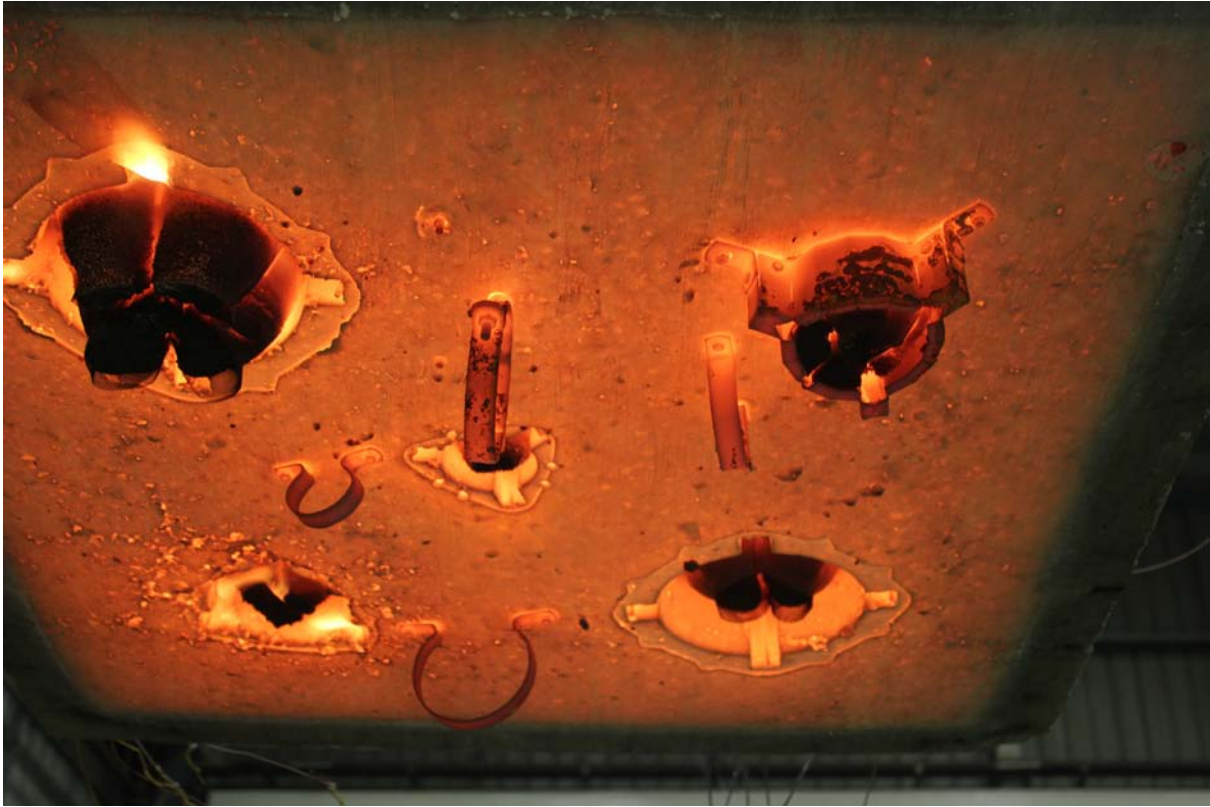
Photograph 7 – Exposed face of the specimens at the conclusion of testing
