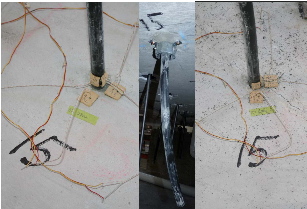
Photo 22: Specimen 16, left to right, unexposed, exposed and unexposed post test
