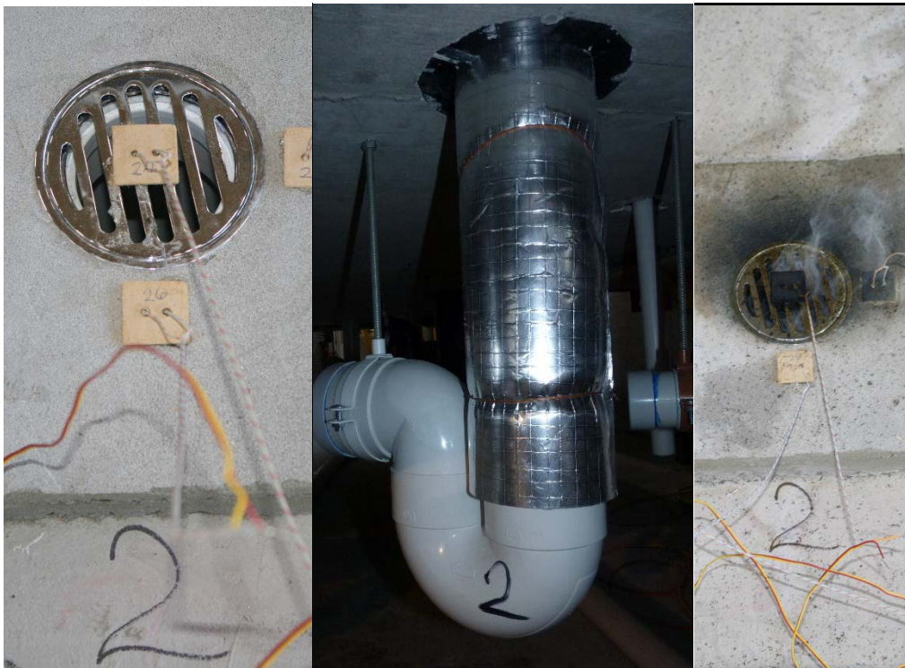
Photo 8: Specimen 2, left to right, unexposed, exposed and unexposed post test
