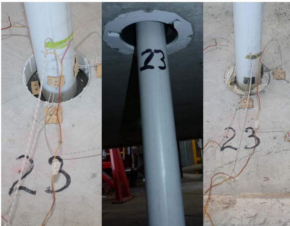
Photo 28: Specimen 23, left to right, unexposed, exposed and unexposed post test
