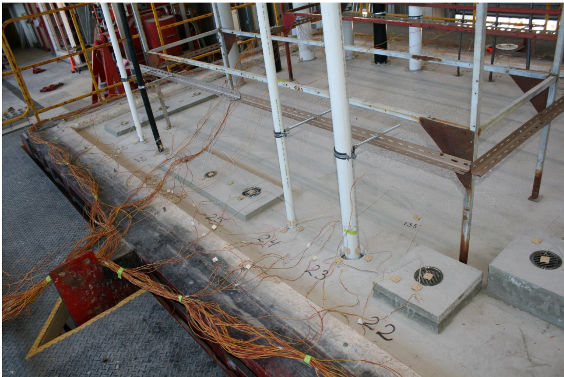
Photo 4: Pre-test unexposed face Specimens 22 to 29
