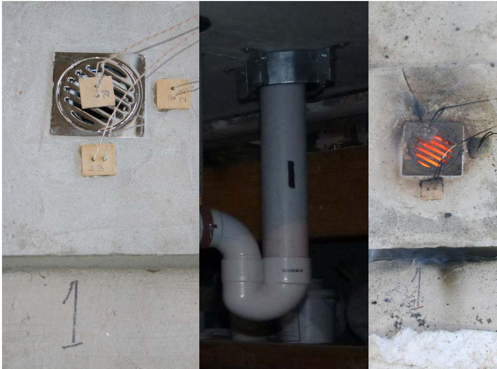
Photo 8: Specimen 2, left to right, unexposed, exposed and unexposed post test
