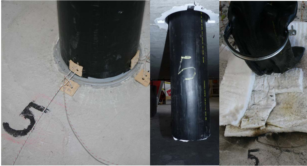
Photo 12: Specimen 6, left to right, unexposed, exposed and unexposed post test
