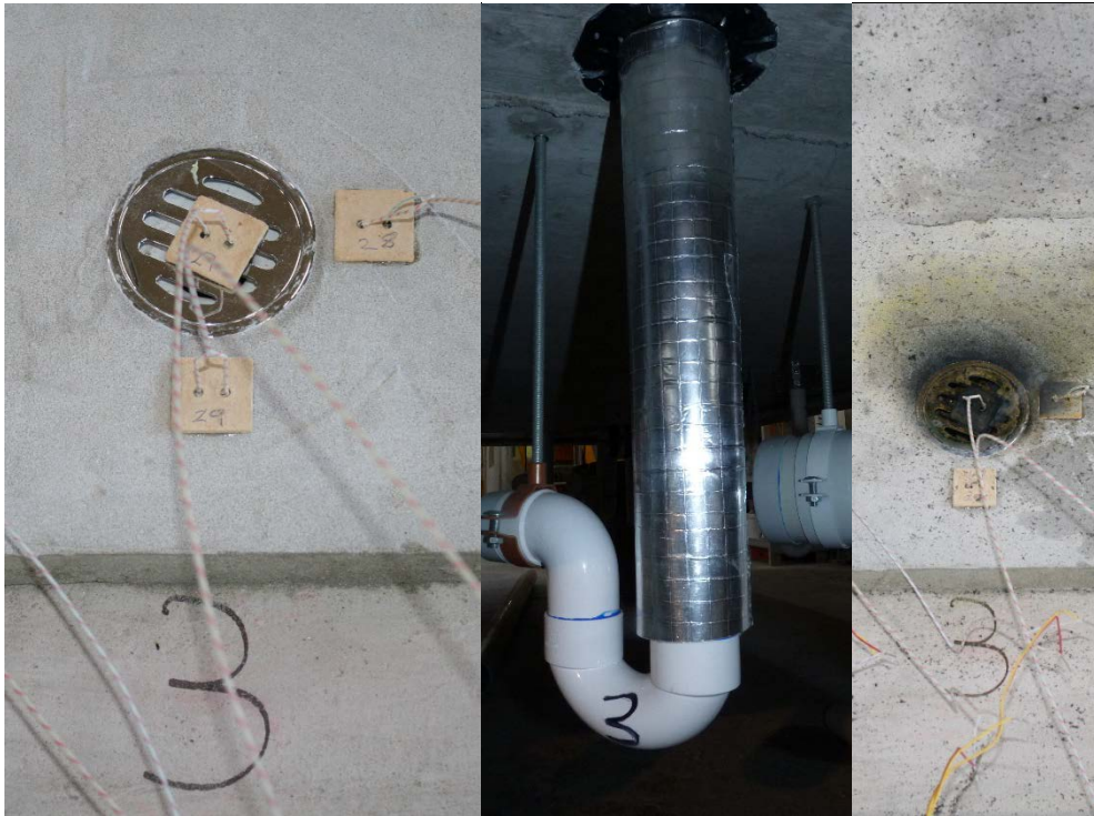
Photo 10: Specimen 4, left to right, unexposed, exposed and unexposed post test
