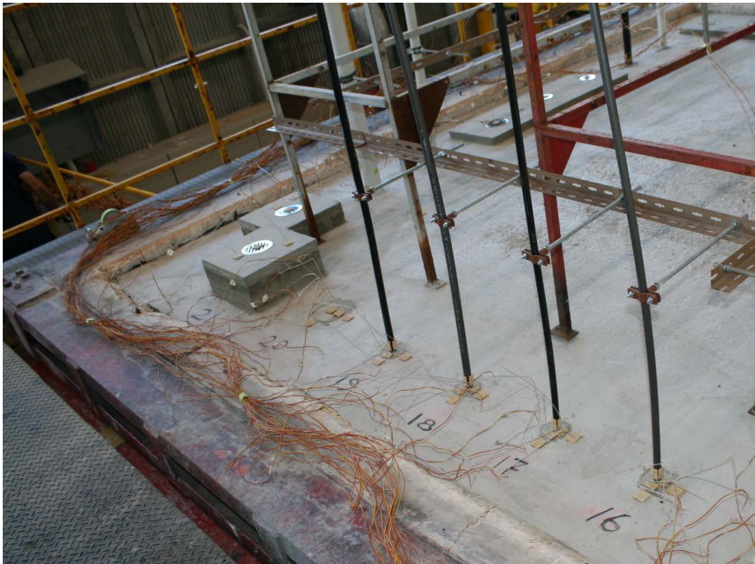
Photo 4: Pre-test unexposed face Specimens 22 to 29
