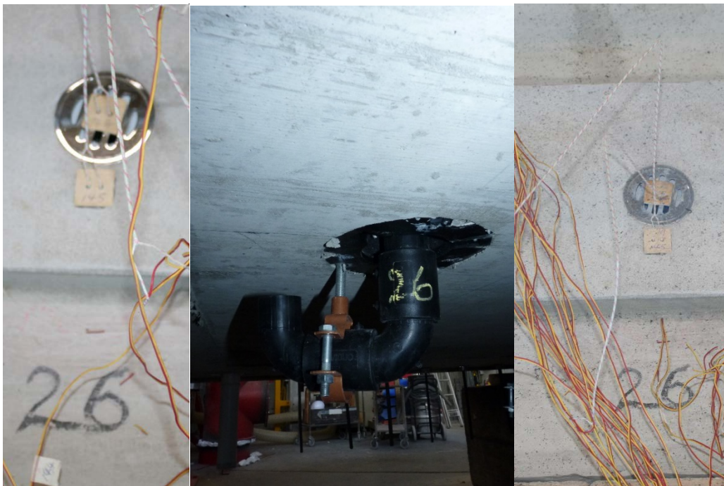
Photo 30: Specimen 26, left to right, unexposed, exposed and unexposed post test
