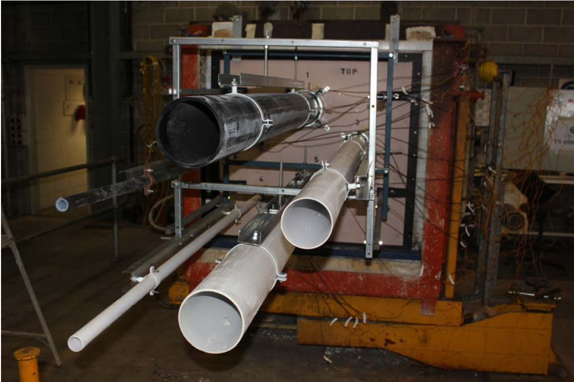
PHOTOGRAPH 1 – UNEXPOSED FACE OF SPECIMENS PRIOR TO TESTING
