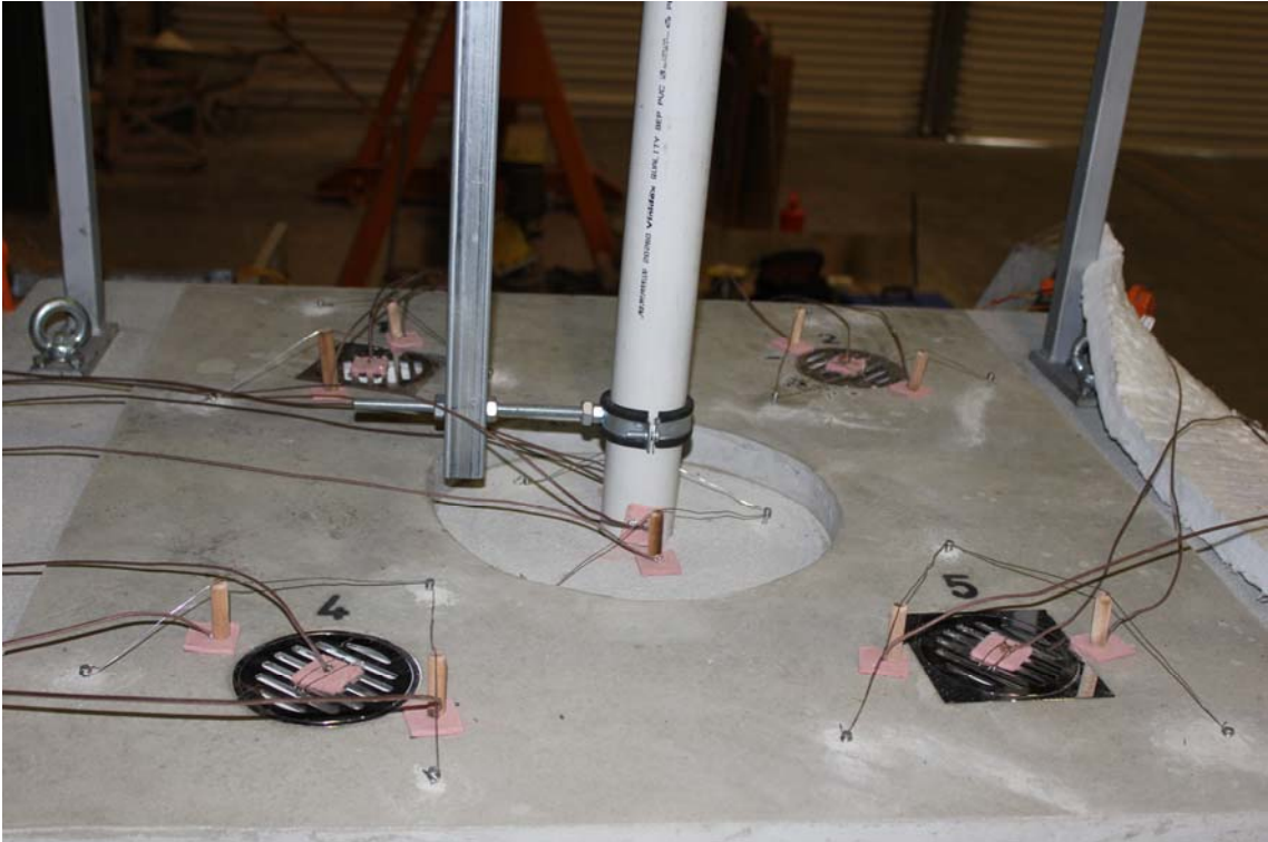
PHOTOGRAPH 2 – UNEXPOSED FACE OF SPECIMENS PRIOR TO TESTING
