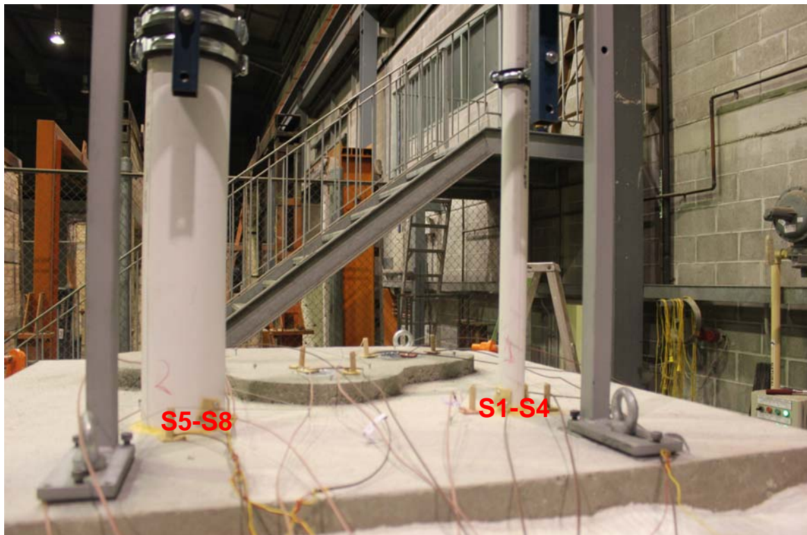
Photograph 2 – Unexposed face of penetrations #1 and #2 prior to testing
