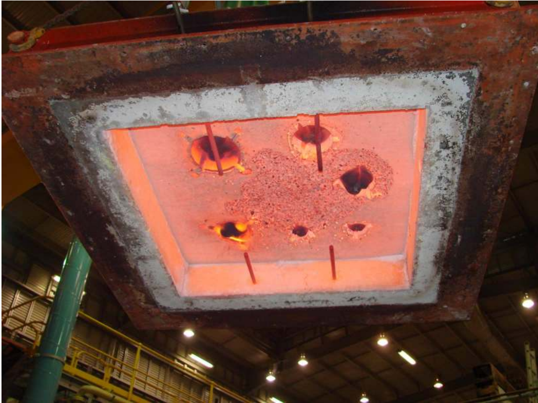
Photograph 9 – Exposed face after the conclusion of testing
