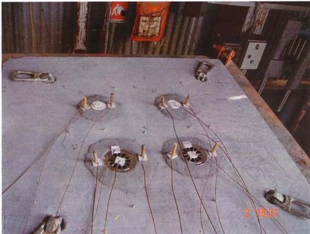
Photograph 2 – Specimens (unexposed side) prior to testing.
