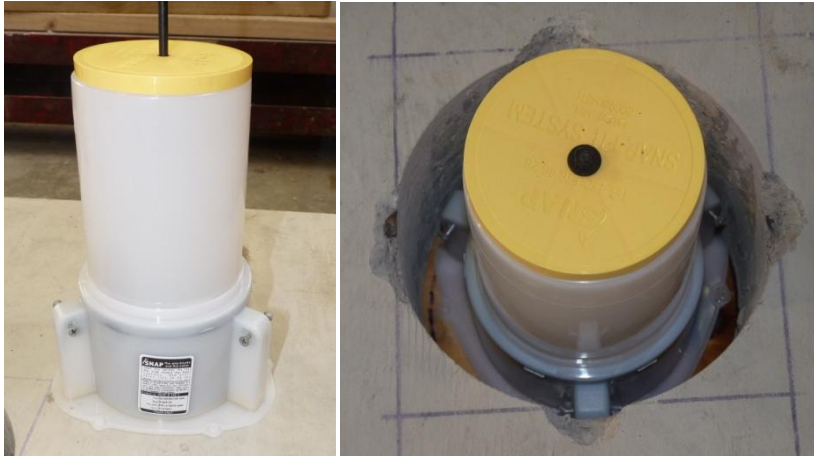
Unexposed Face after grouting
