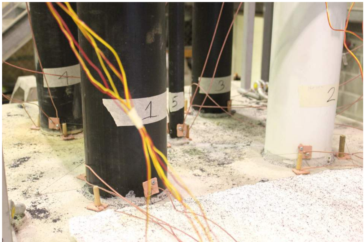
PHOTOGRAPH 4 – SPECIMENS AFTER 120 MINUTES OF TESTING
