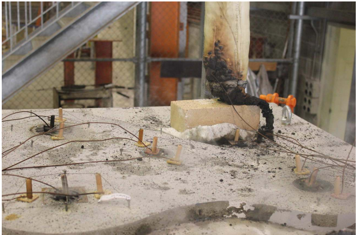
Photograph 4 – Specimens after 120 minutes of testing
